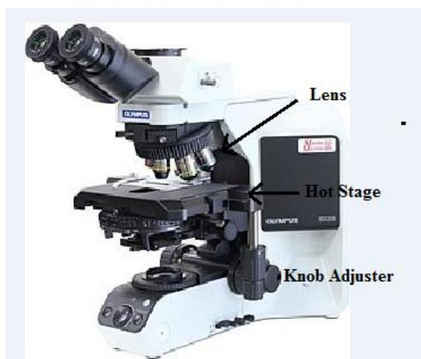
Figure 3.6: Cross-Polarised Microscope BX53
