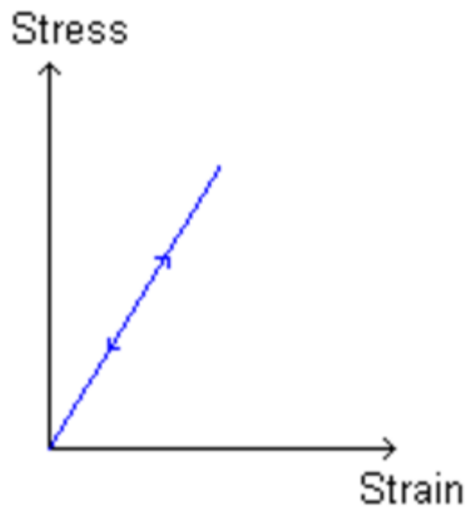
Figure 4.4: Stress-strain curve of an isotropic linear elastic material (Atkinson, n.d.)
