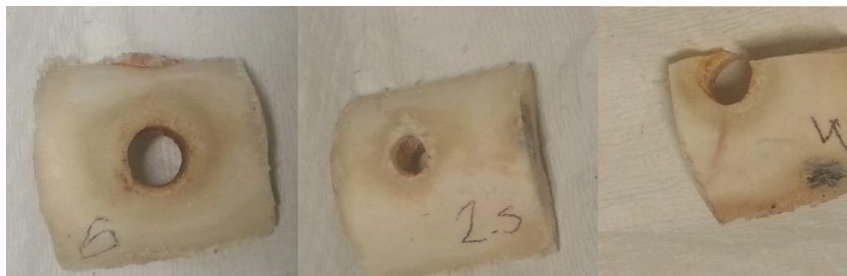
Figure 4.3: 5mm, 2.5mm and 4mm drilled specimens
