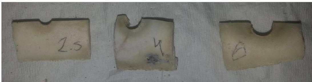
Figure 4.4: Specimens were cut in half to test surface roughness
