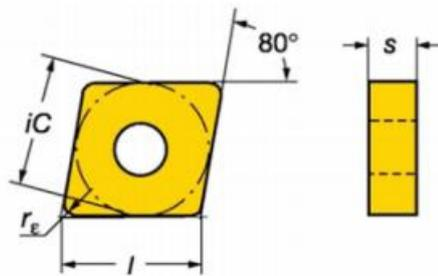
**Figure 3 : Schematic geometry of the insert used in the machining**
