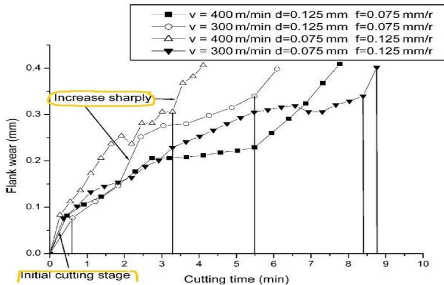
Graph 1 - The tool wear evolution in different working conditions .
