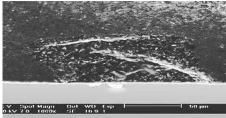
**Figure 14 SEM views of Plastic Deformation (V = 200 m/min, feed = 611.4mm/min)**
