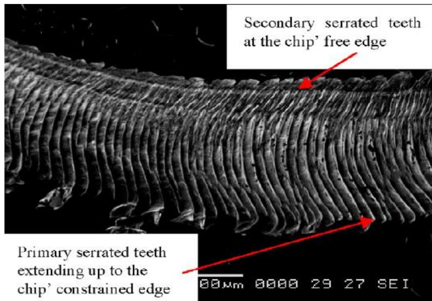
**Figure 18 SEM micrographs of chip's top view for uncoated carbide inserts: (a) at 120m/min.**
