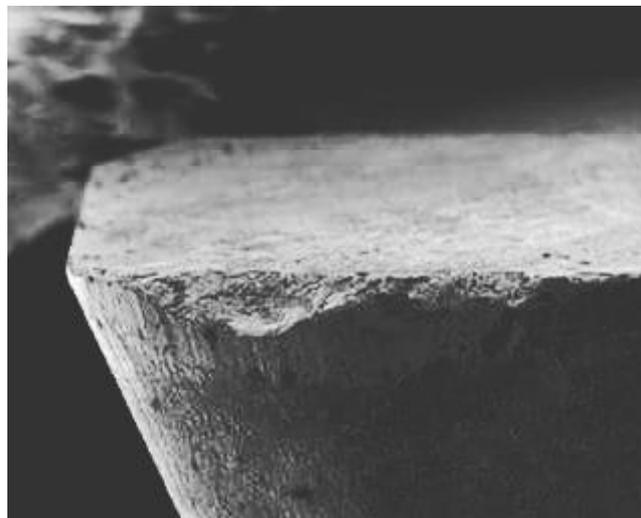
**Figure 15 SEM views of Diffusion (V = 160 m/min, feed = 488.83mm/min)**
