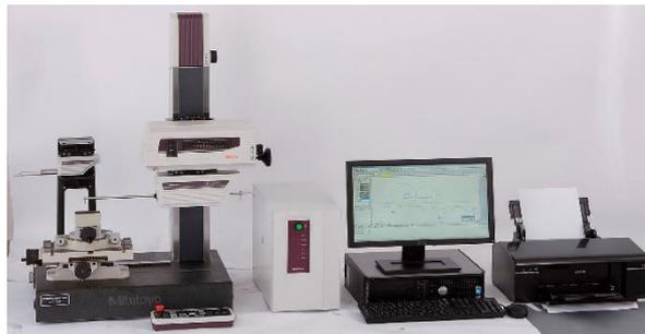
**Figure 10 Surface Roughness Machine**
