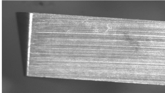
**Figure 16 SEM views of the WC–Co inserts before machining experiments.**
