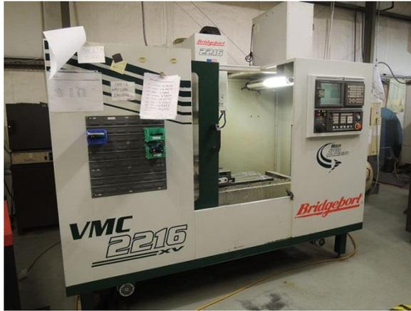
**Figure 9 CNC Milling machine**
