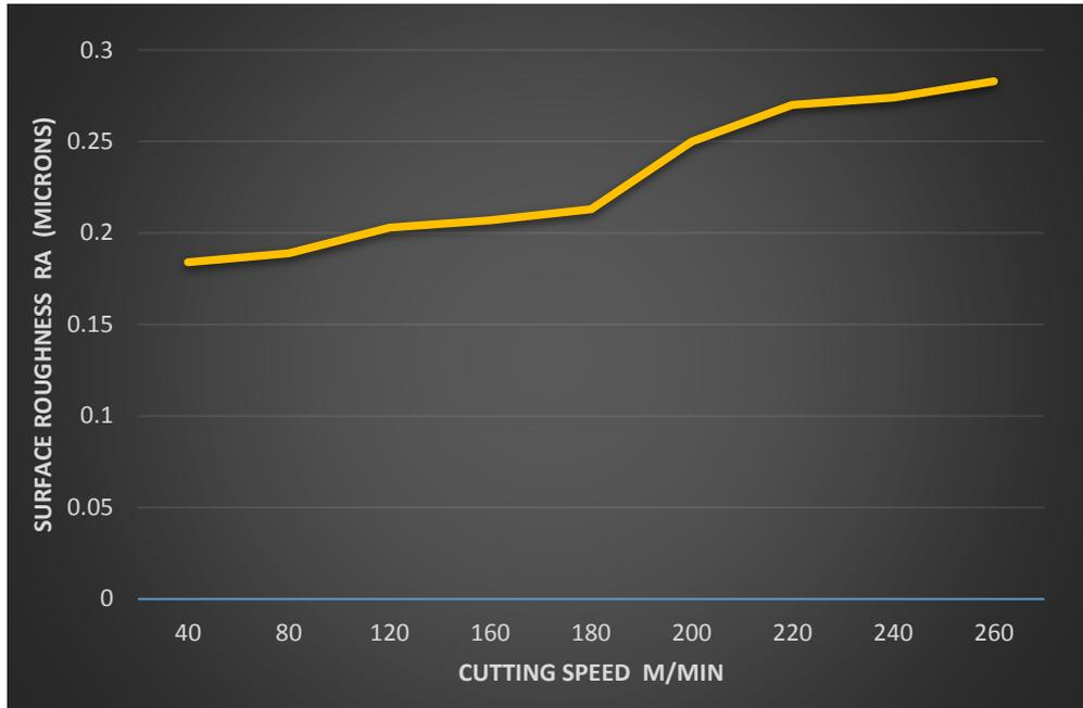
**Graph 5 Surface Roughness vs Cutting speed**
