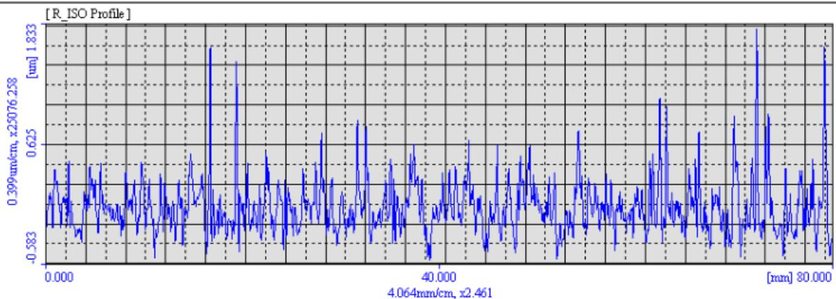
(Cutting speed 80 m/min , feed 244.420 mm/min, depth of cut 0.2 mm)
