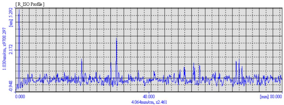
(Cutting speed 180 m/min , feed 550.10 mm/min, depth of cut 0.2 mm)
