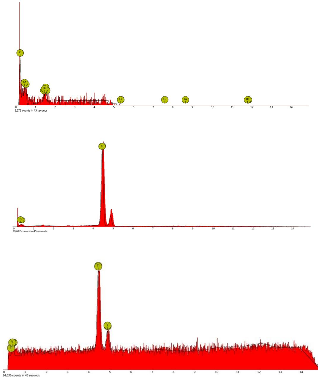
**Graph 3 EDS spectrum of chips at 120 ,160 and 240 m/min respectively**
