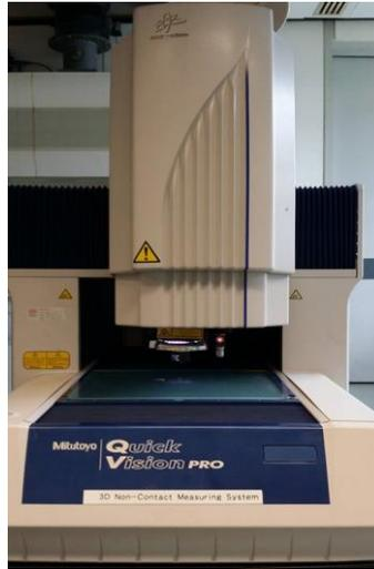
**Figure 11 3D Non- Contact Measuring Machine**
