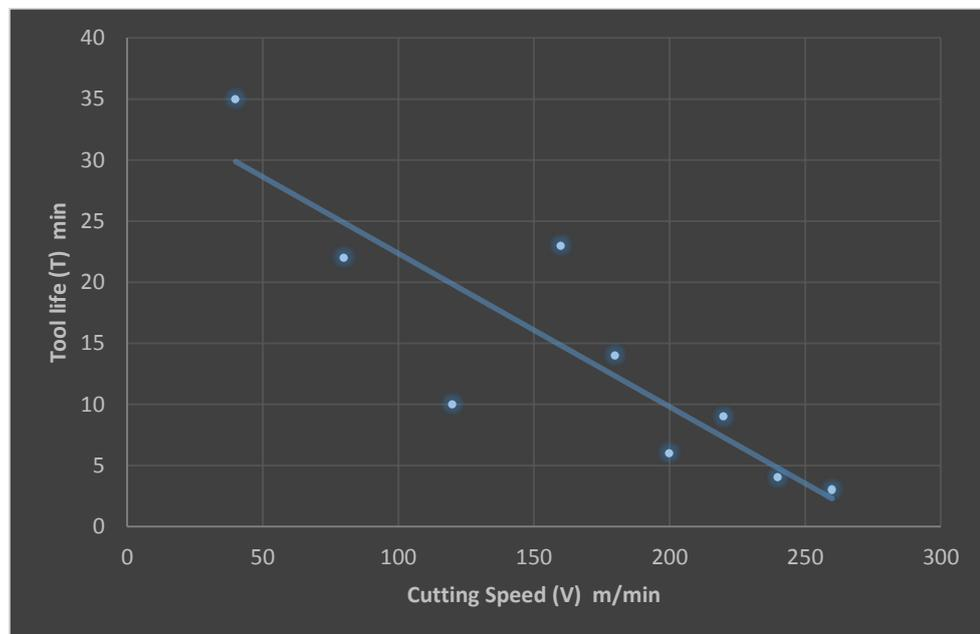
**Fig. 12 Tool life curve for uncoated carbide inserts**
