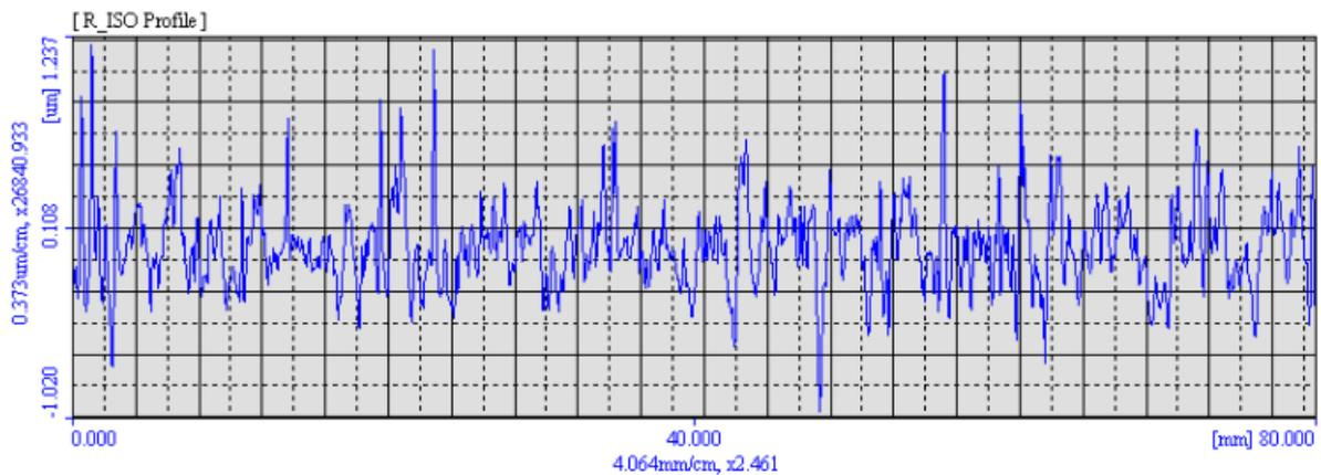
(Cutting speed 40m/min , feed 122.304 mm/min, depth of cut 0.2 mm)
