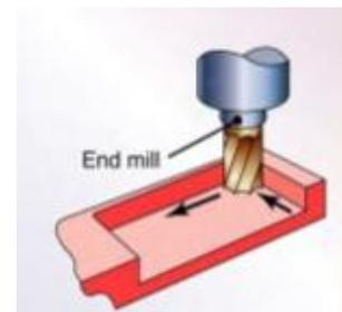
**Figure 1** End milling of titanium
