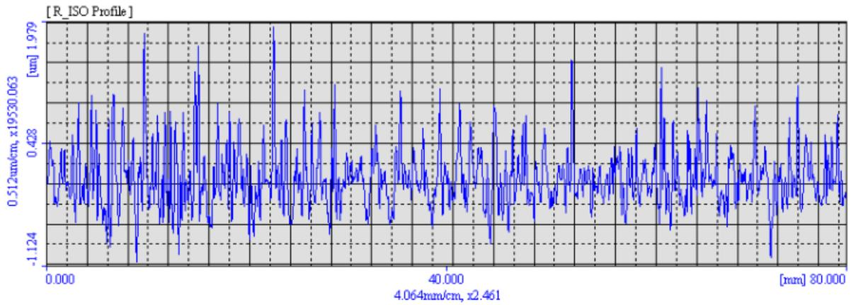
(Cutting speed 240m/min , feed 733.44 mm/min, depth of cut 0.2 mm)
