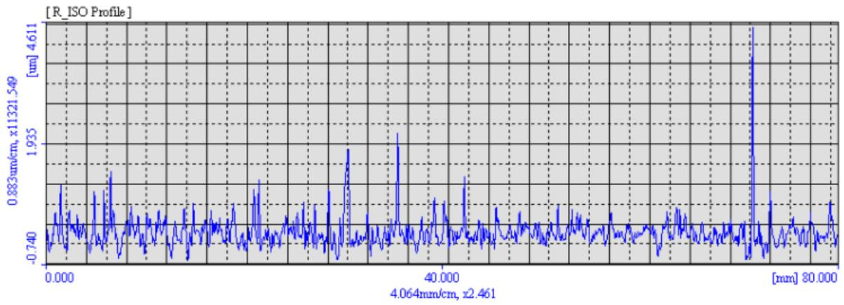
(Cutting speed 120 m/min , feed 366.72 mm/min, depth of cut 0.2 mm)
