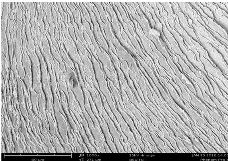
**Figure 20** SEM micrographs of chip's top view for uncoated carbide inserts at 160m/min
