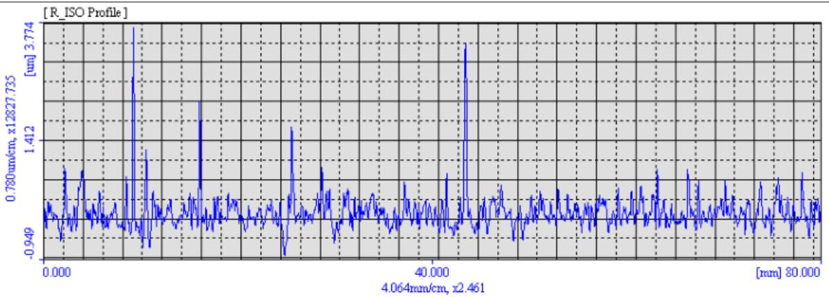
(Cutting speed 160 m/min , feed 488.832 mm/min, depth of cut 0.2 mm)
