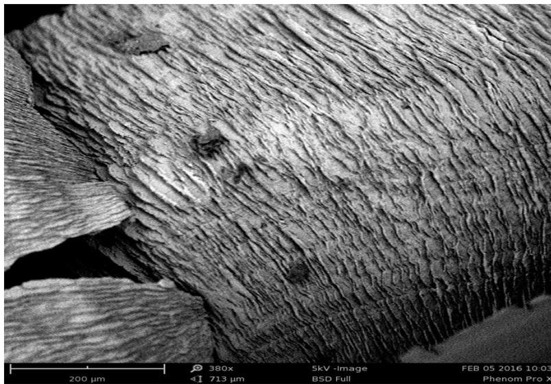
**Figure 22** SEM micrographs of chip's top view for uncoated carbide inserts at 220 m/min
