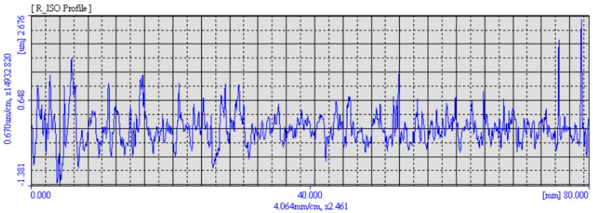
(Cutting speed 260 m/min , feed 794.50 mm/min, depth of cut 0.2 mm)
