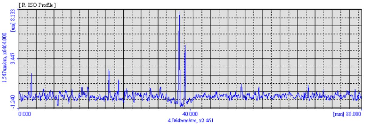
(Cutting speed 220 m/min , feed 672.193 mm/min, depth of cut 0.2 mm)
