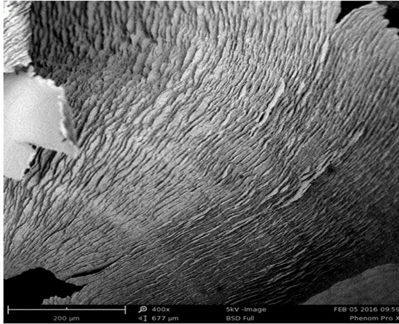
**Figure 19** SEM micrographs of chip's top view for uncoated carbide inserts at 100m/min
