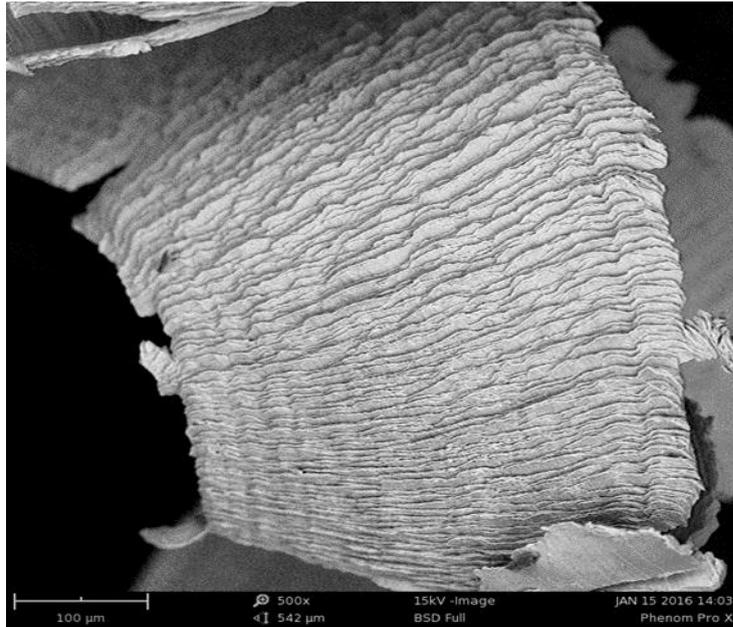
**Figure 21** SEM micrographs of chip's top view for uncoated carbide inserts at 180 m/min
