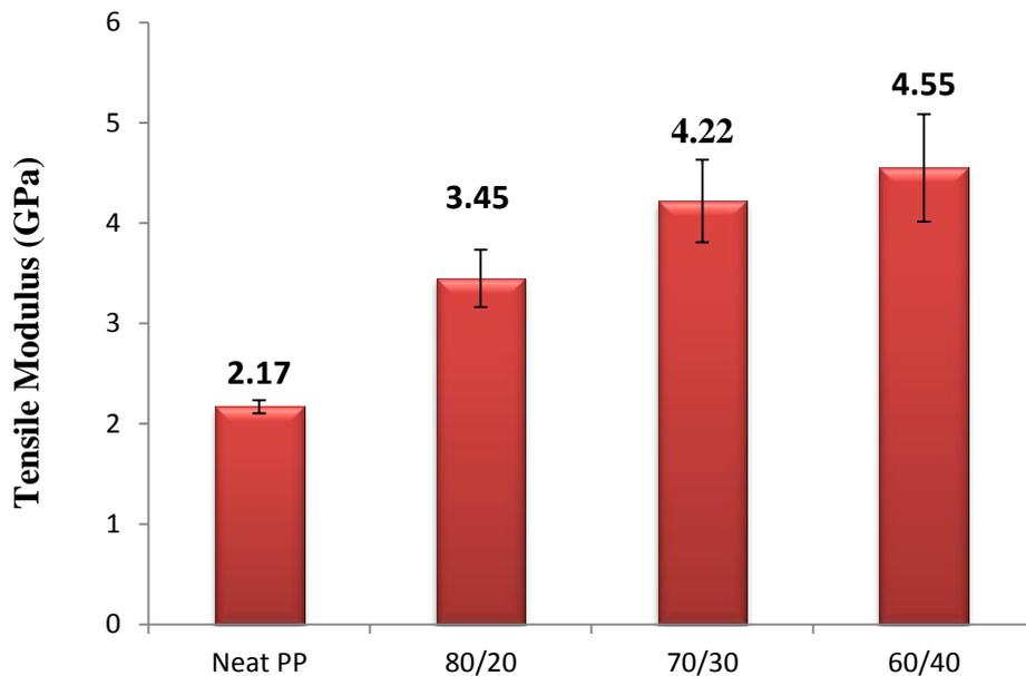
Figure 4.3: Tensile modulus of neat PP and mengkuang fibre reinforced PP composite.
