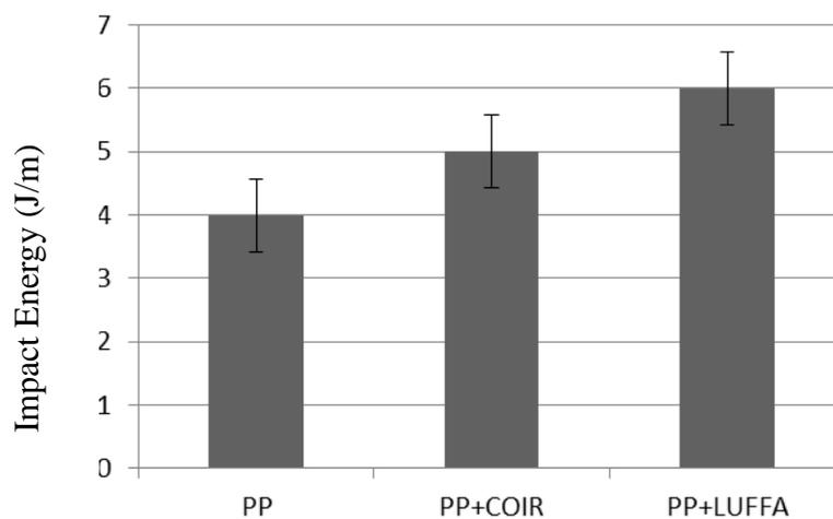
Figure 2.3: Impact energy of coir and luffa fibre reinforced polypropylene composite [12].
