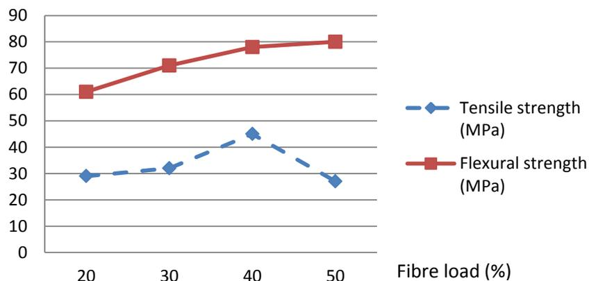
Figure 2.6 Tensile and flexural strength of abaca fibre reinforced polypropylene [15].
