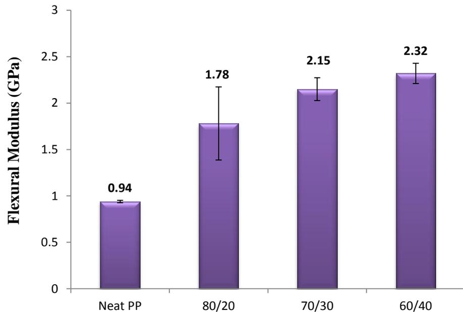
Figure 4.5: Flexural modulus of neat PP and impact energy of mengkuang fibre and PP composites.
