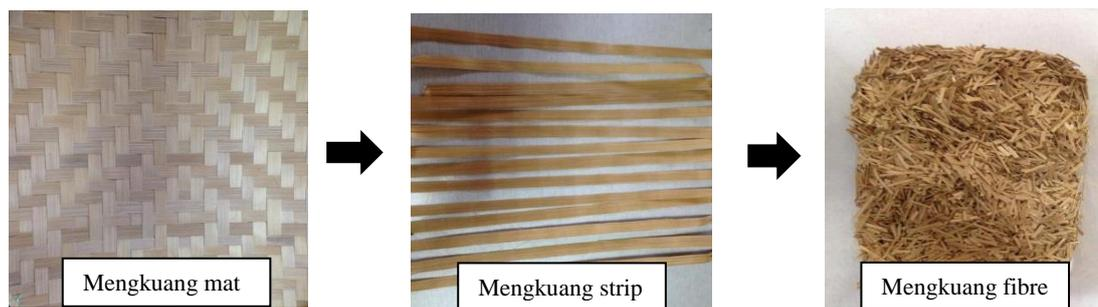
Figure 3.2: Sequence of mengkuang fibre preparation.
