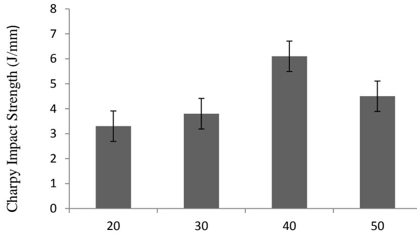
Figure 2.7: Impact strength of abaca fibre reinforced polypropylene [15].
