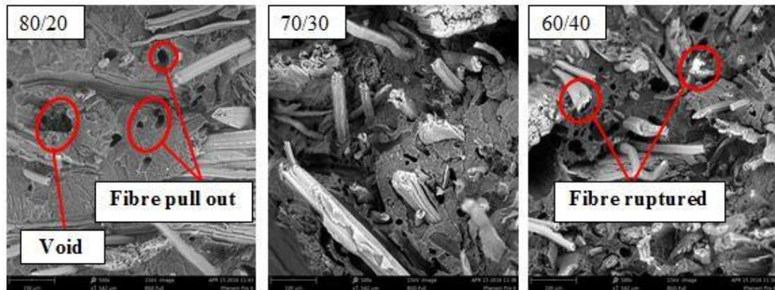
Figure 4.2: SEM micrographs of PP/mengkuang fibre composite with different compositions
