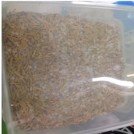
Figure 3.3: Sample mixture of mengkuang fibre and PP granules.
