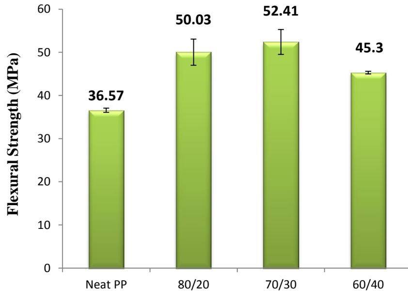
Figure 4.4: Flexural strength of neat PP and impact energy of mengkuang fibre and PP composites.
