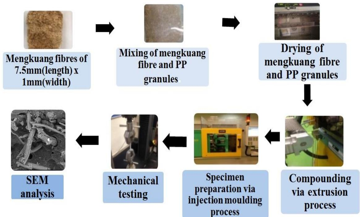
Figure 3.1: Process flow diagram of main activities.
