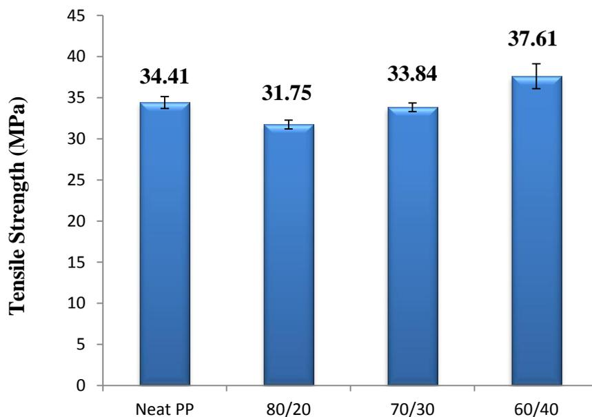
Figure 4.1: Tensile strengths of neat PP and mengkuang fibre reinforced PP composite.
