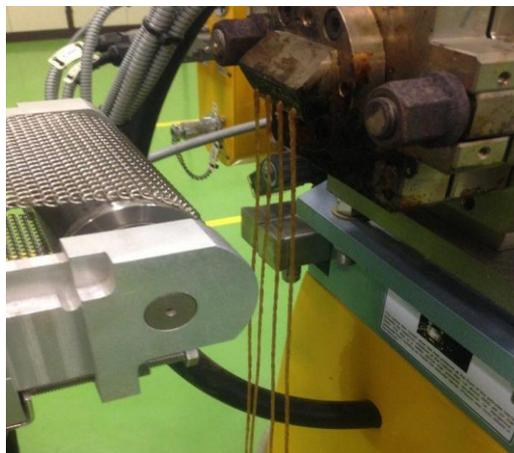
Figure 3.4: Extrudate PP/mengkuang fibre composite.
