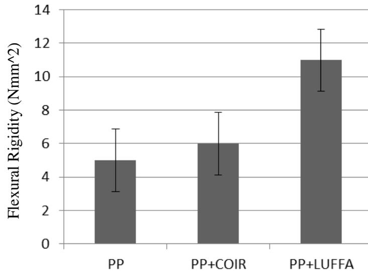
Figure 2.2: Flexural rigidity of coir and luffa fibre reinforced polypropylene composite [12].
