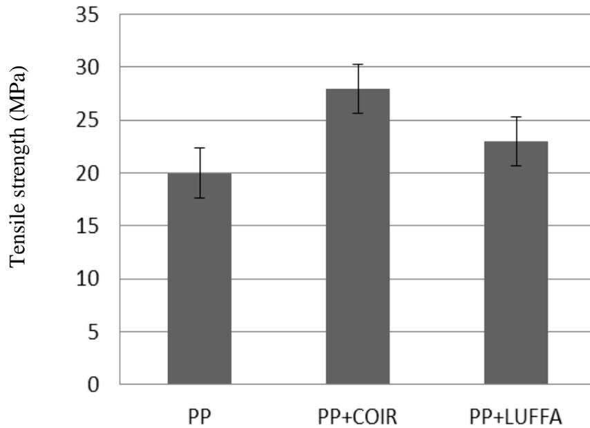
Figure 2.1: Tensile strength of coir and luffa fibre reinforced polypropylene composite [12].
