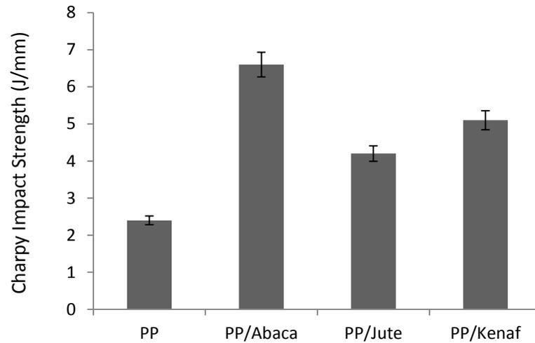
Figure 2.5: Charpy impact strength of abaca, jute, kenaf fibre reinforced polypropylene composite [13].
