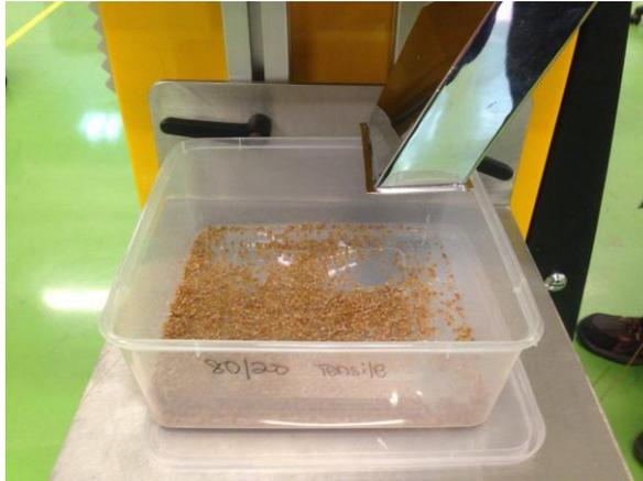
Figure 3.5: Pellets of PP/mengkuang fibre composite.
