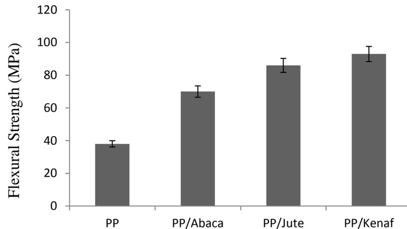
Figure 2.4: Flexural strength of abaca, jute, kenaf fibre reinforced polypropylene composite [13].
