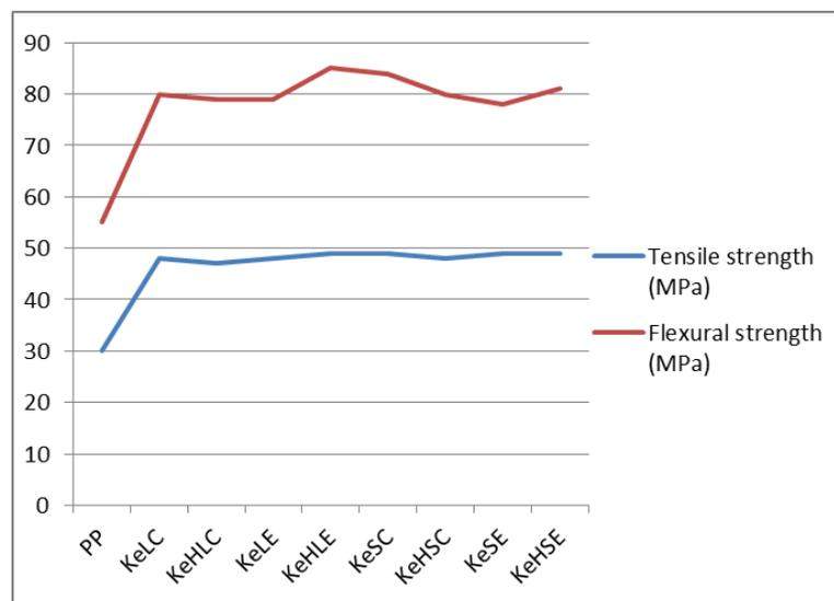
Figure 2.8: Tensile and flexural properties of polypropylene reinforced kenaf composites [17].
