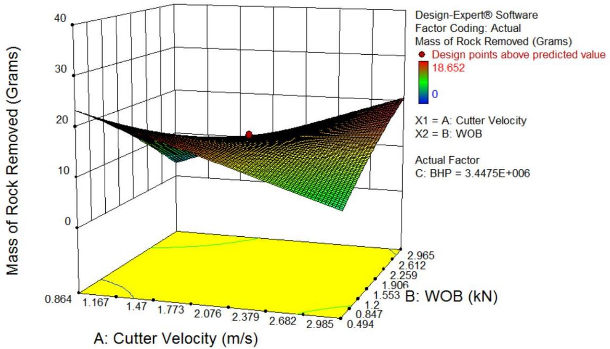
Figure 14: Response Surface for Rock Removed Mass (Factor = BHP@3.4475E+06, Mean)
