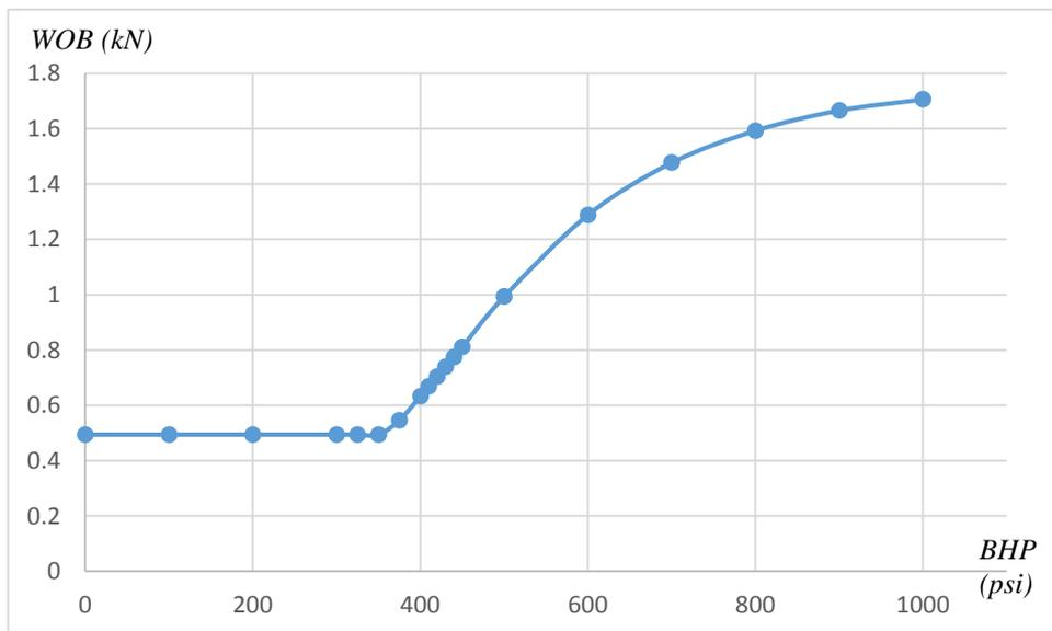
Figure 17: Optimum Cutter WOB for Varying Bottom Hole Pressure
