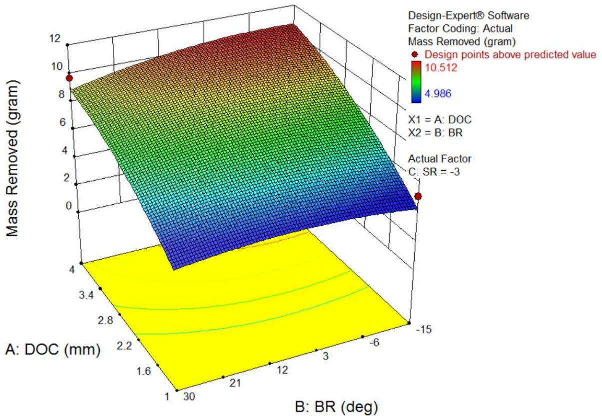
Figure 10: Response Surface for Mass Removed (Actual Factor = Side Rake @ -3°)
