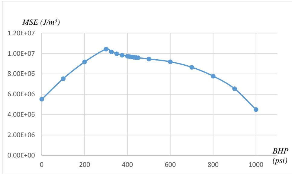
Figure 18: MSE Response for Varying Bottom Hole Pressure
