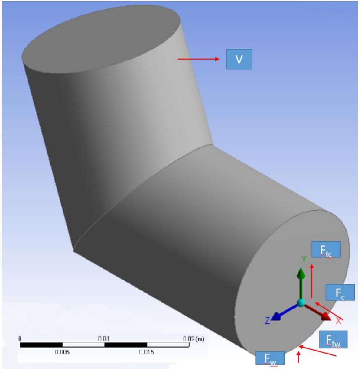
Figure 4: Free Body Diagram of a Single PDC Cutter and Forces Acting on It
