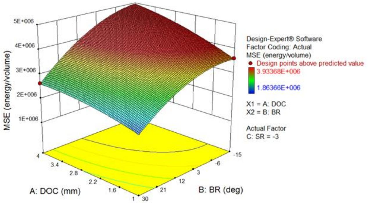
Figure 9: Response Surface for MSE (Actual Factor = Side Rake @ -3°)
