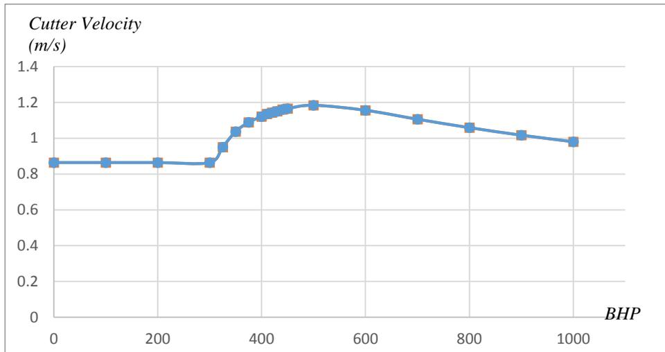
Figure 16: Optimum Cutter Velocity for Varying Bottom Hole Pressure
