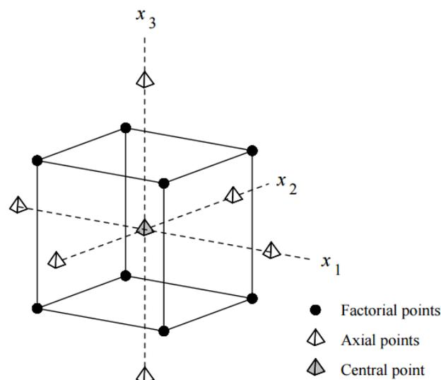
Figure 1: CCD for 3 design variables at 2 levels
