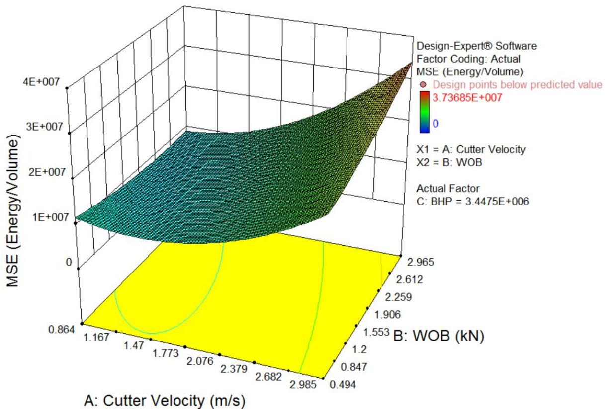
Figure 13: Response Surface for MSE (Actual Factor = BHP@3.4475E+06, Mean)
