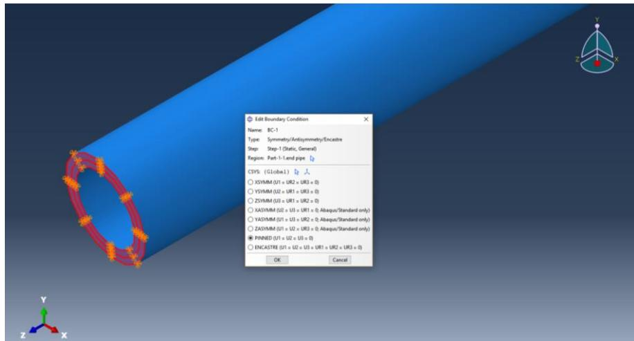
FIGURE 12 Both end pipe boundary conditions
