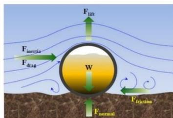
FIGURE 3. Forces Acting on Pipeline [3]
