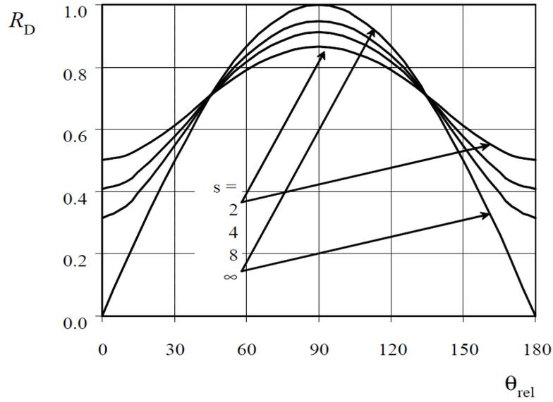
FIGURE 9. Reduction factor due to wave spreading and directionality [11]
