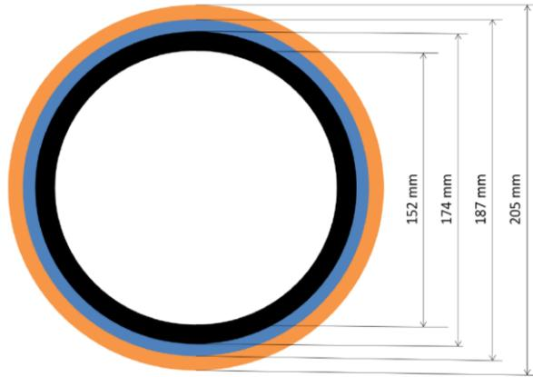
FIGURE 6. Non-Metallic Pipeline by AIRBORNE
