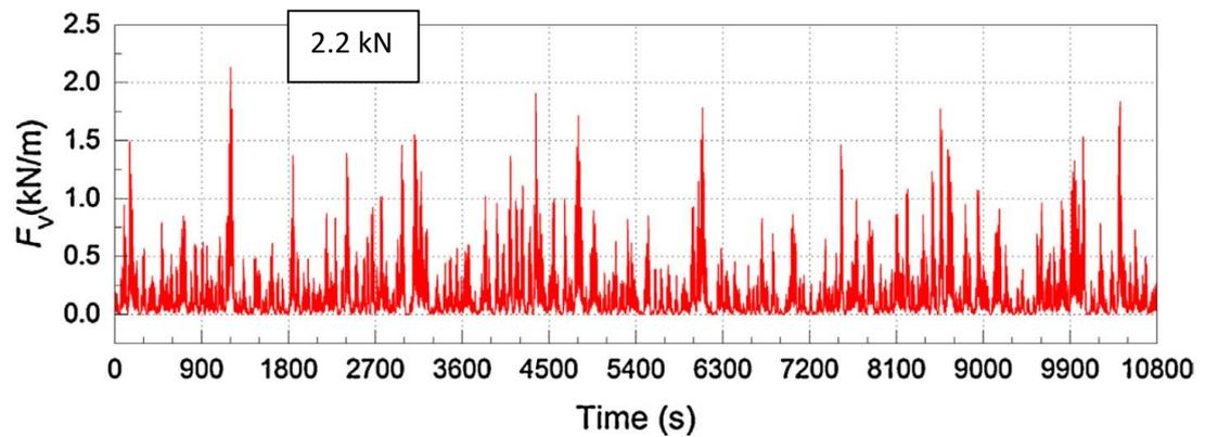
FIGURE 29 Times series of Vertical forces over 10800s at the pipeline midpoint from ABAQUS Subroutine
