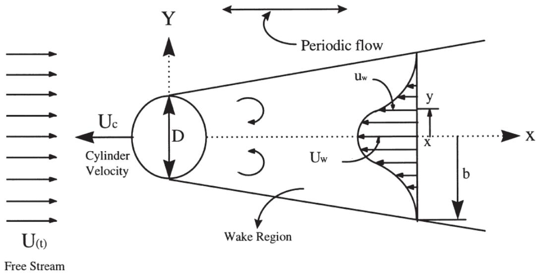
FIGURE 7. Velocity flow on pipeline on the seabed [18]
