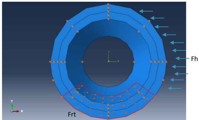
FIGURE 13 Soil resistance as surface traction on the pipeline
