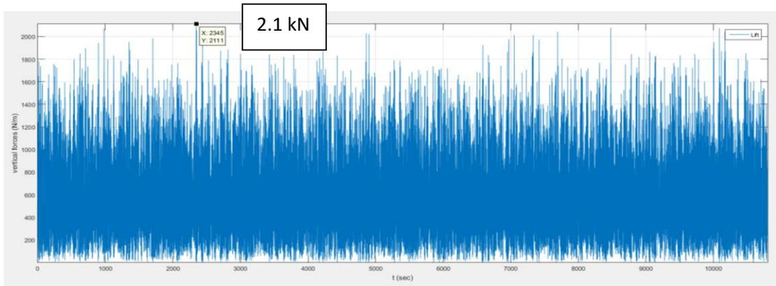
FIGURE 28. Time series of Vertical forces over 10800s from MATLAB at pipeline midpoint
