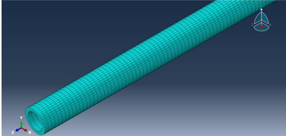
FIGURE 11 Pipeline meshing
