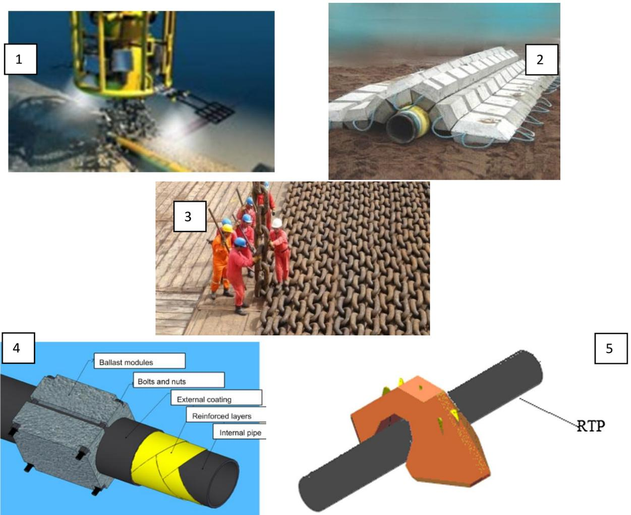
FIGURE 4. Offshore RTP anchoring methods (1-rock dumping, 2- concrete mattress, 3-chain, 4-rock bolts and 5-gravity anchor) [3]
