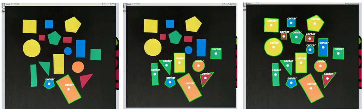
Figure 21: Step by step detection of center contour
