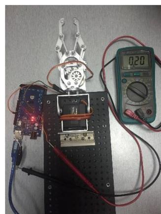
Figure 16: Current needed by Servo Motor (Gripper System)
