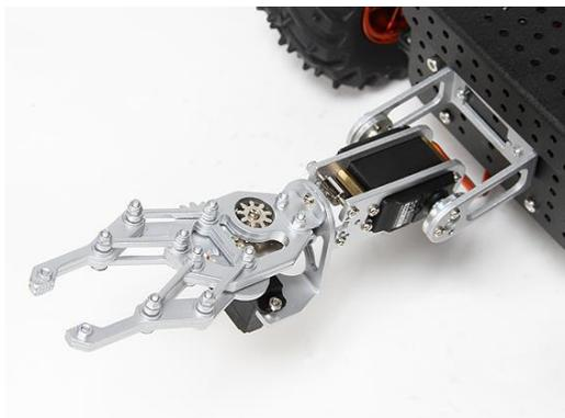
Figure 13: Gripper Mechanism
