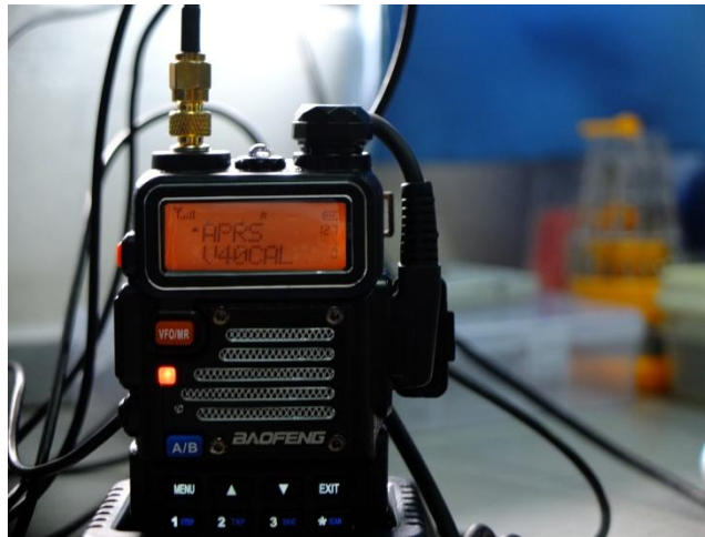
Figure 20 VHF transceiver is set at APRS channel 144.390MHz
