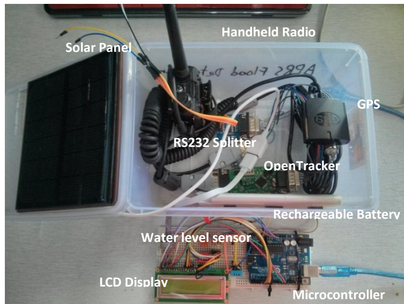
Figure 35 APRS Flood monitoring Prototype
