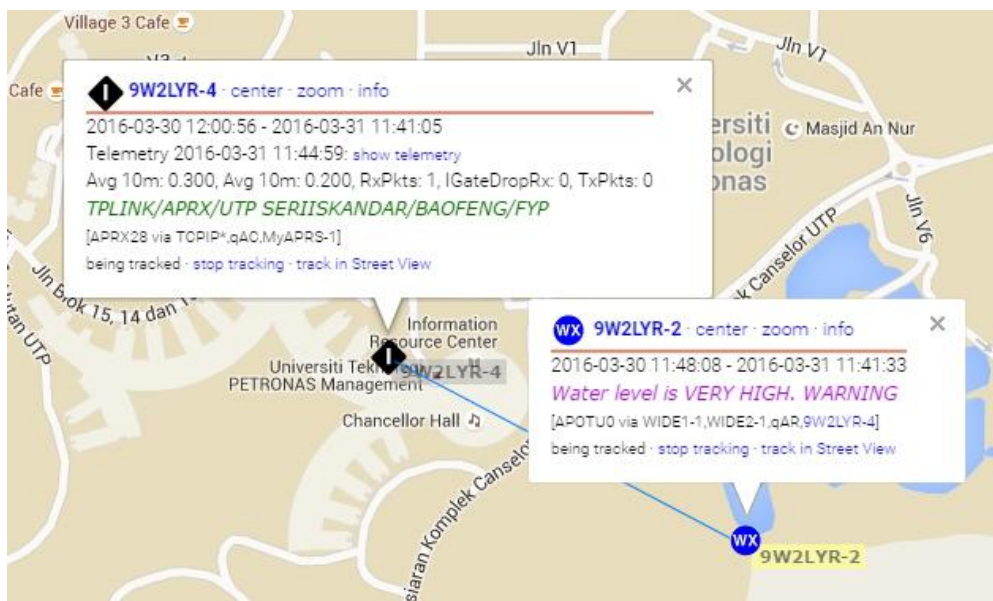
Figure 33 Monitor the warning status at APRS.FI using internet browser
