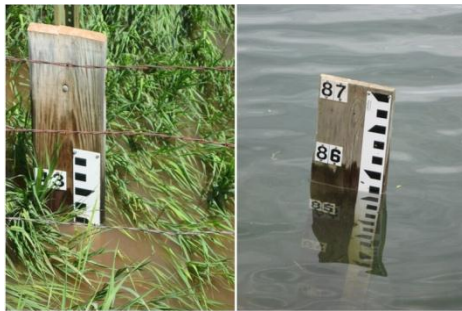
Flood monitoring old system.
