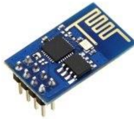
FIGURE 6. ESP8266 Wi-Fi module
