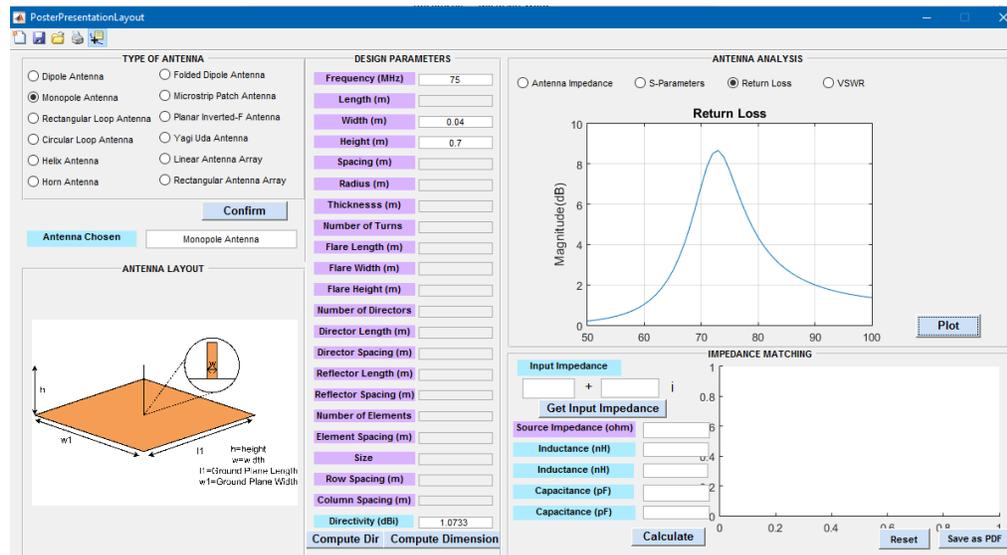
Figure 27: Return loss graph is plotted
