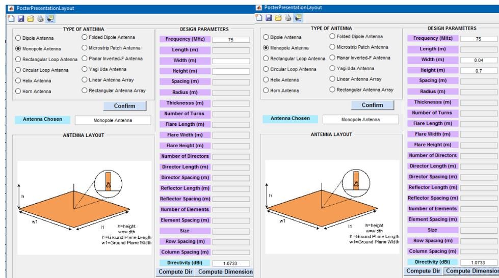
Figure 25: (a) Directivity is defined. (b) Antenna dimension is calculated.
