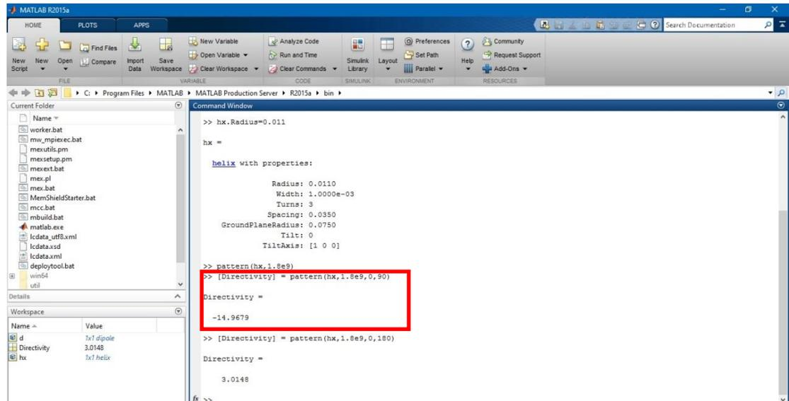
Figure 14: Directivity of antenna calculated with the azimuth and elevation as well as the frequency prompted from user
