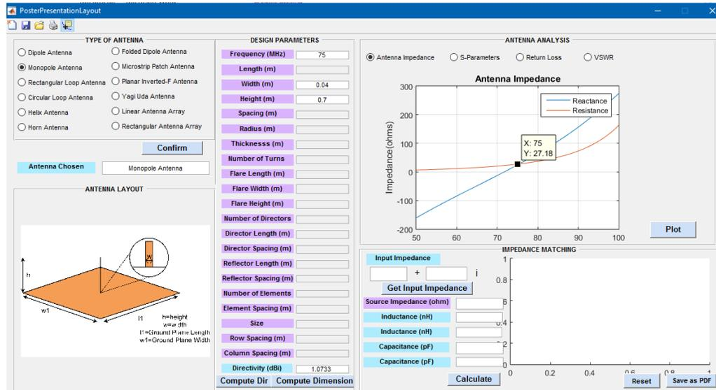
Figure 26: Antenna Impedance graph is plotted
