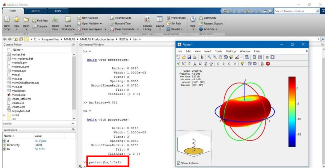
Figure 13: Radiation Pattern of Antenna with Frequency Input by User
