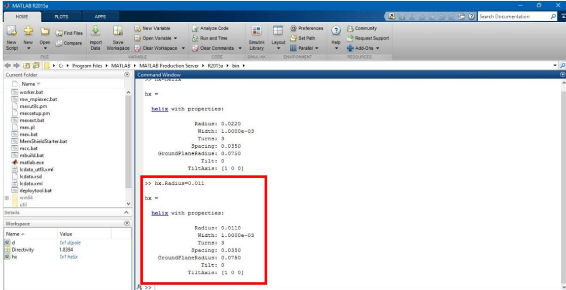
Figure 12: Properties of antenna can be modify easily
