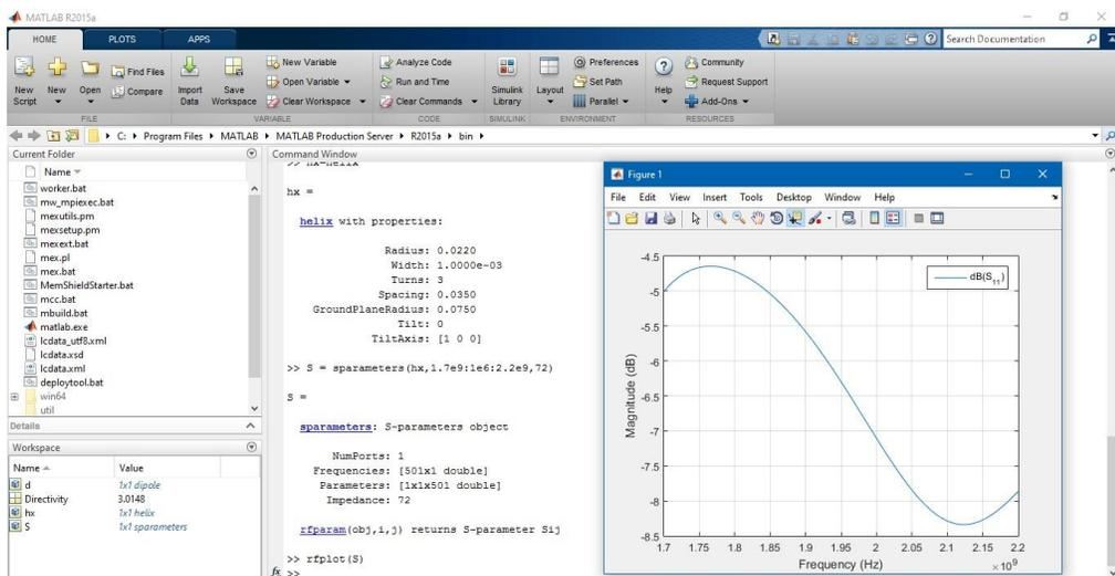
Figure 17: Reflection Coefficient Graph
