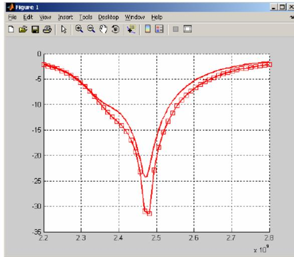
Figure 5: Result of antenna return loss simulated by MAT (squared curve) and return loss predicted by ANSOFT HFSS (solid curve)
