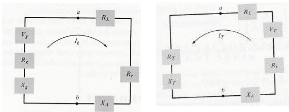
Figure 4: Thevenin equivalent of antenna in transmitting and receiving mode
