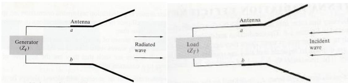
Figure 3: Antenna system in transmitting and receiving mode
