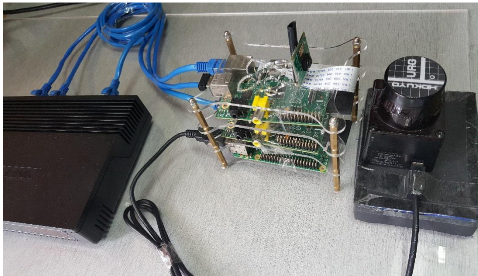
Figure 23: LRF and camera setup
