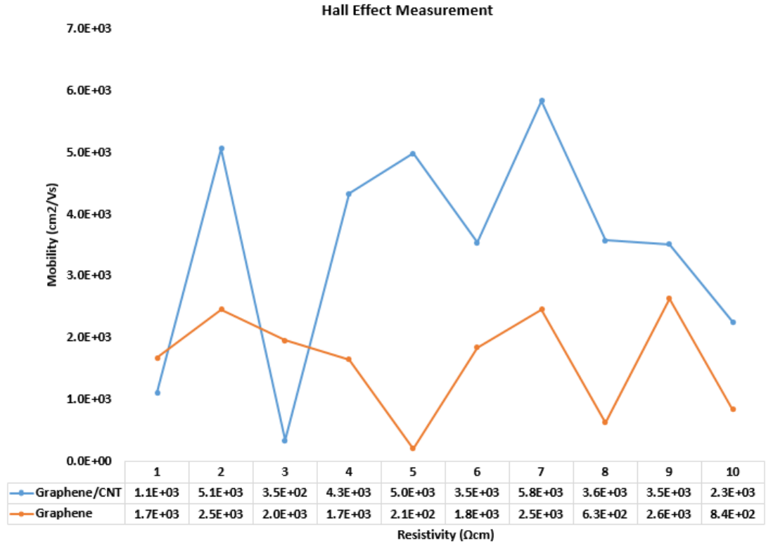
Figure 16. Mobility vs Resistivity of Graphene and Graphene-CNT.
