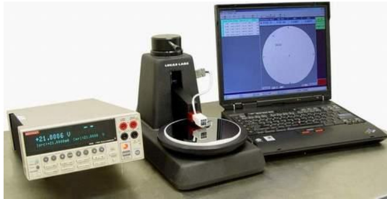
Figure 13: 4 Point Probing System
