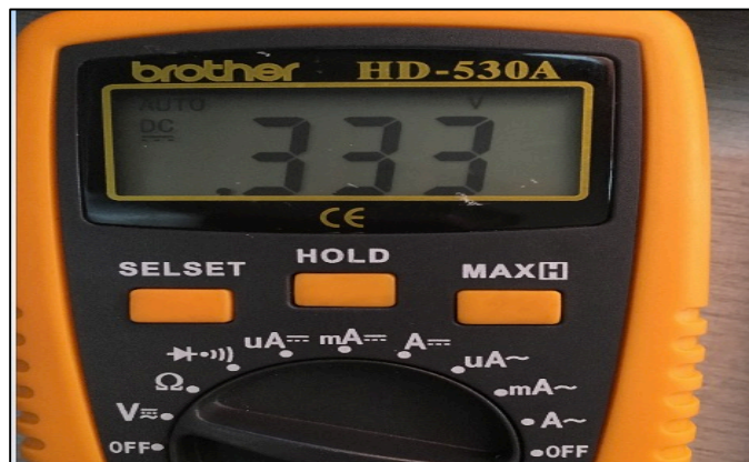
FIGURE 4.3 Measured voltage output from LM35 temperature sensor
