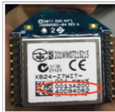
FIGURE 3.4 XBee Coordinator 64-bit serial number
