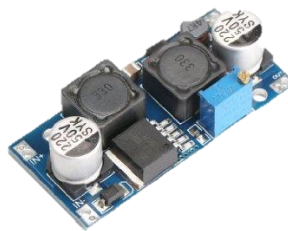
FIGURE 13: 5A dc-to-dc boost-buck converter
