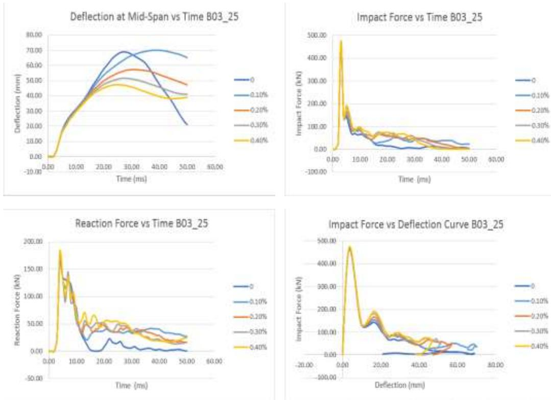
Figure 5. Graphs of the impact responses with respect to shear reinforcement ratio exhibited by the beam models with  $a/d$  ratio = 3 and with main reinforcements of 2T25.
