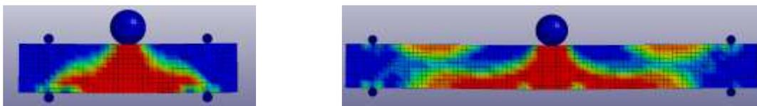
Figure 8. Plot of effective strain distribution in LS-DYNA for beam models with a/d ratio = 2 and 5 respectively.
