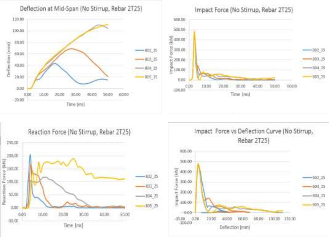
Figure 6. Graphs of the impact responses with respect to a/d ratio exhibited by the beam models without shear reinforcements and with main reinforcements of 2T25.
