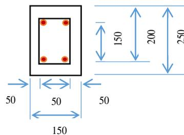
Figure 2. Details of the arrangement of reinforcement bars: Cross-sectional view, unit = mm.
