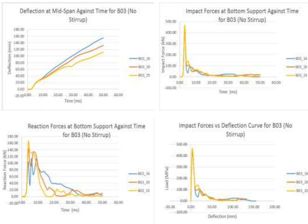
Figure 3. Graphs of the impact responses exhibited with respect to longitudinal reinforcement ratio by the beam models with a/d ratio = 3 and without shear reinforcement
