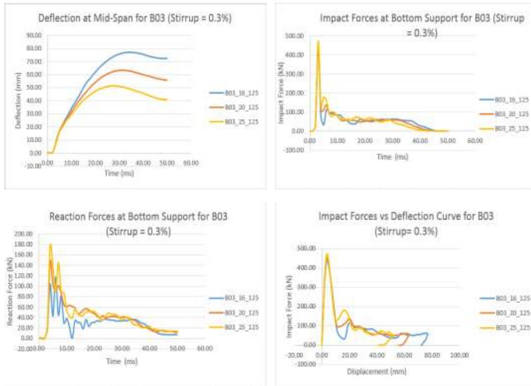
Figure 4. Graphs of the impact responses exhibited with respect to longitudinal reinforcement ratio by the beam models with a/d ratio = 3 and with shear reinforcement ratio of 0.3%
