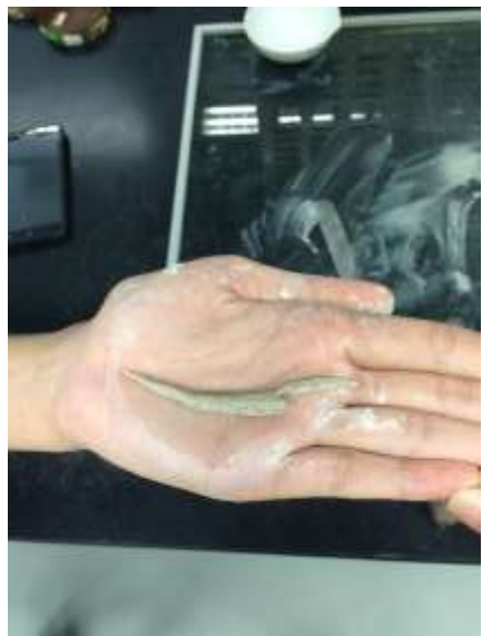
The sample is rolled into thin pieces to find the plastic limit
