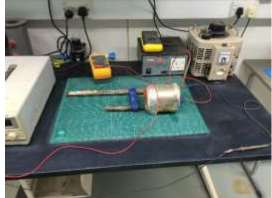
The setup for electrical resistivity test
