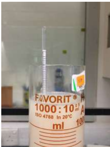
The hydrometer reading is taken at 30s, 1min, 2min, 4min, 8min, 15min, 30min, 1h, 2h, 4hr and 24hr
