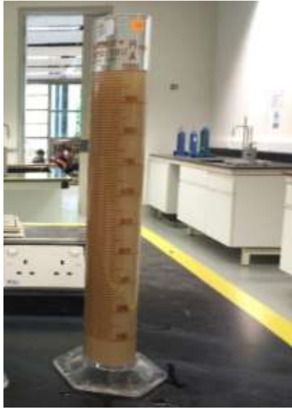
The material passing the 63 \mu\text{m} sieve is added in the measuring cylinder and distilled water is added up to 1L mark
