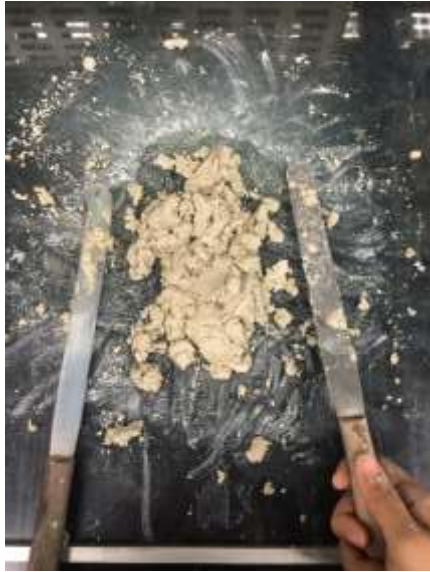
The sand and silt is mixed together using spatula and distilled water is added
