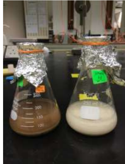
100g sand/ 50g silt is added into the mixture
