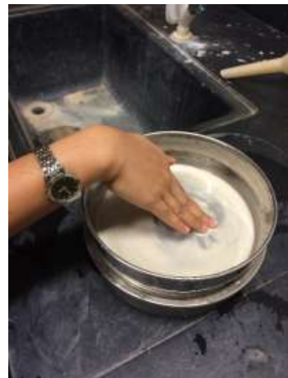
The mixture is massaged on 63 \mu m sieve
