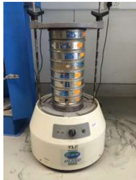
The remaining material that did not pass the 63 \mu\text{m} sieve will be dried in the oven. Sieve analysis is done on the dried material
