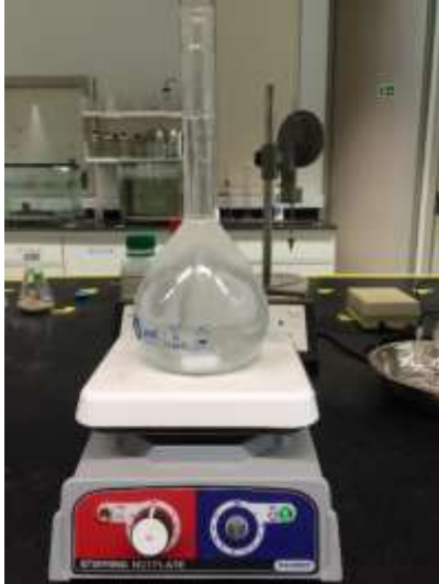
Mixture of sodium carbonate anhydrous, sodium hexametaphosphate and distilled water is being mixed
