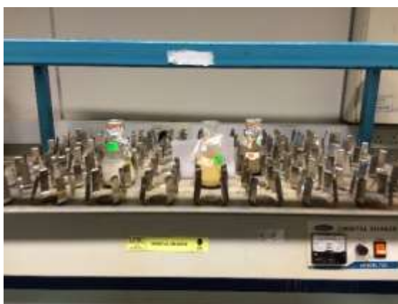
The mixture is left to be shaken for 24 hours in the shaker
