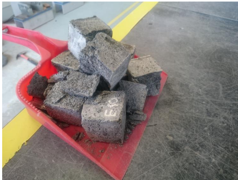
Figure 22: Crushed mortar cubes
