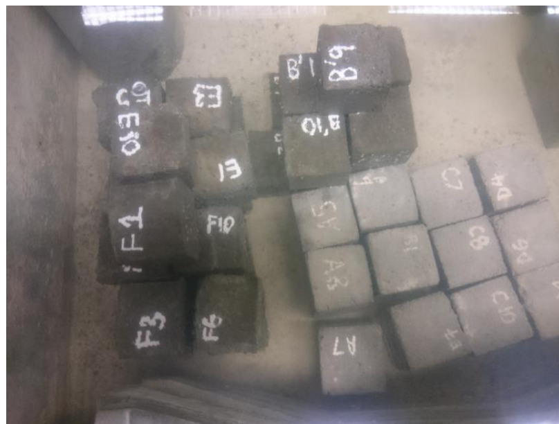
Figure 20: Curing of mortar cubes in curing tank
