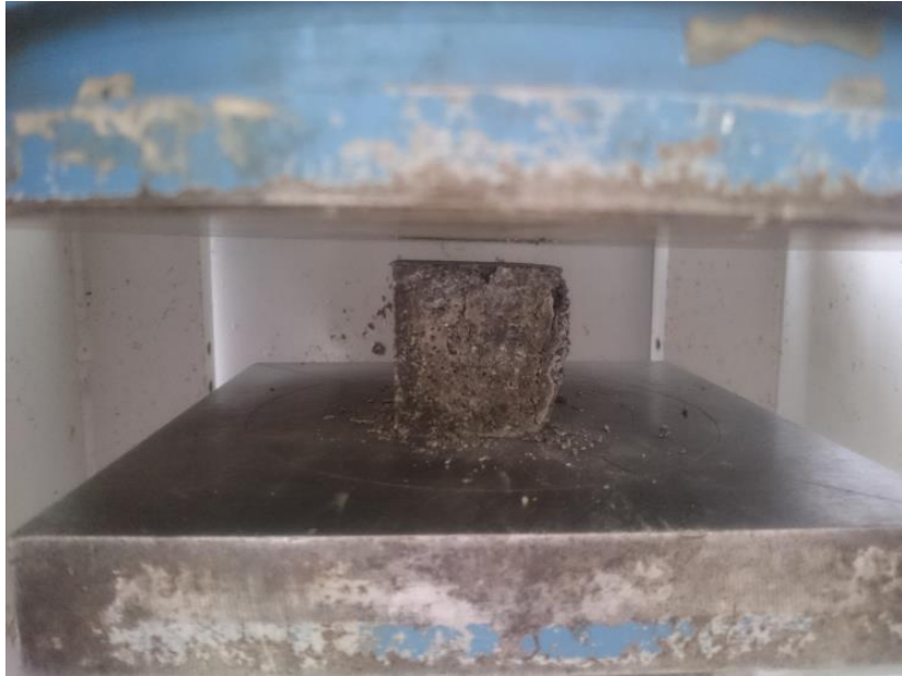
Figure 21: Compressive strength test of the mortar
