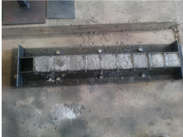
Figure 19: Mortar casted into mold
