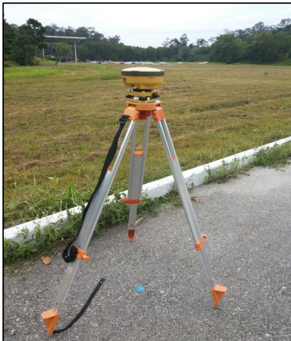
Figure 3.6: Base GPS mounted on tripod
