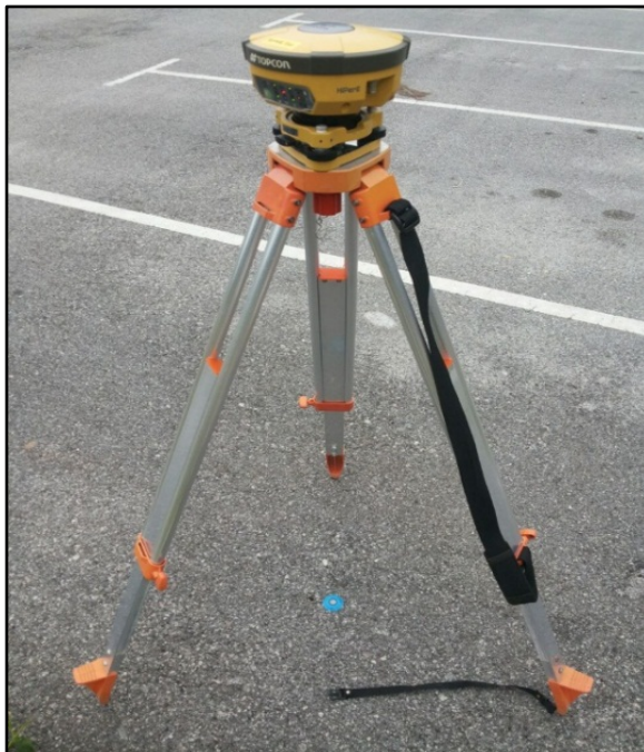
Figure 3.4: Base GPS mounted on tripod
