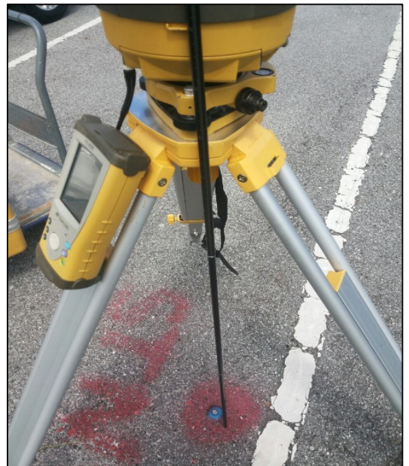
Figure 3.5: Vertical measurement by using measuring rod
