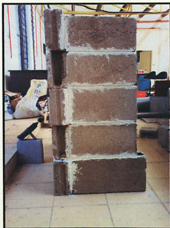
Figure 3.29: Actual side view of the sound reduction testing setup (with side wall)
