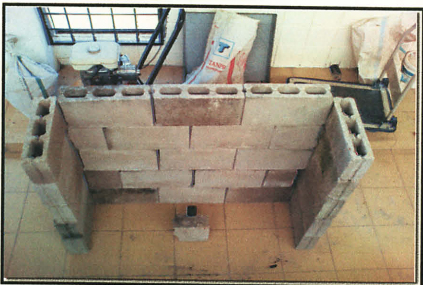
Figure 13.14: Completed prototype crumb rubber noise barrier wall without crumb rubber filler but with side wall
