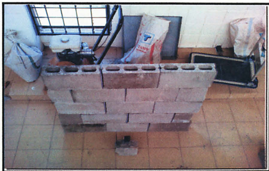
Figure 3.12: Completed prototype crumb rubber noise barrier wall without crumb rubber filler and side wall
