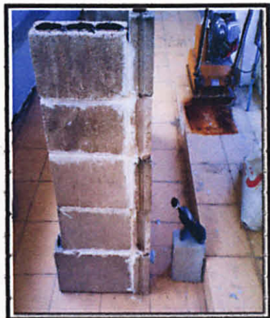
Figure 4.9: Measuring noise behind wall for the right end
