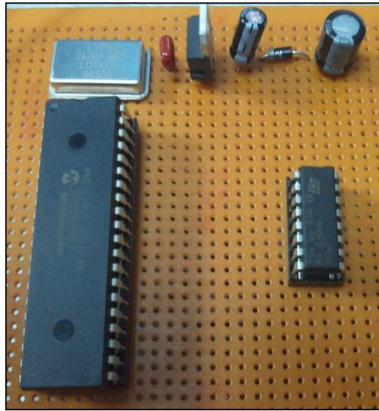
Figure 24: PIC, L239D, and voltage regulator
