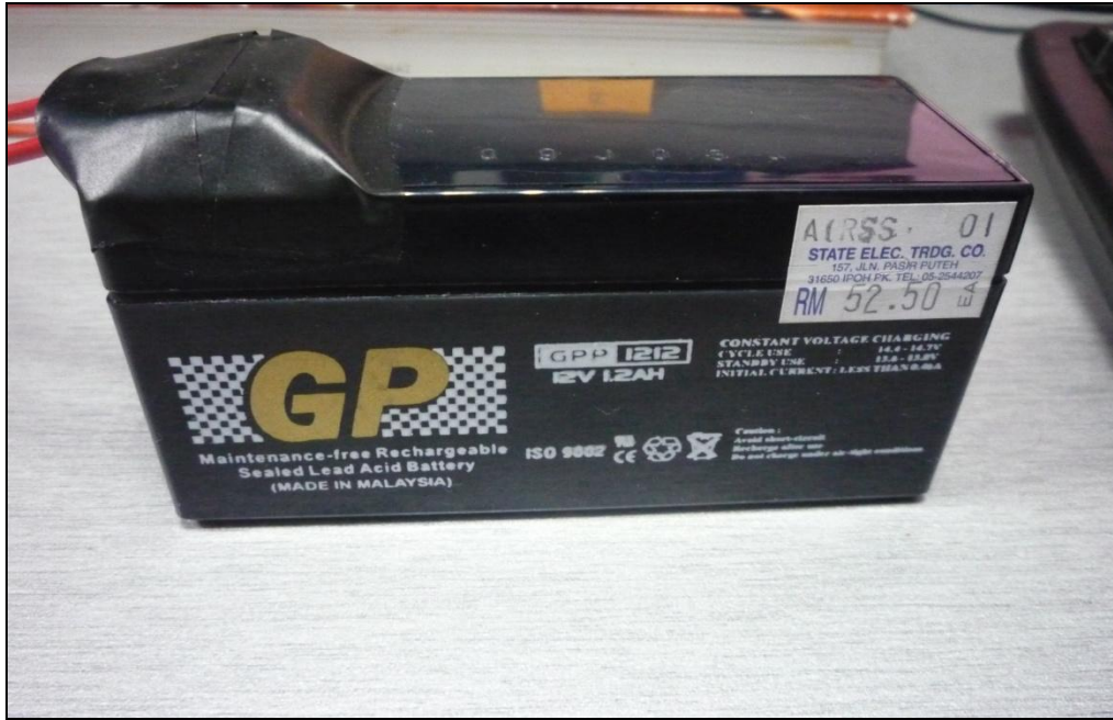
Figure 28: 12V battery lead acid
