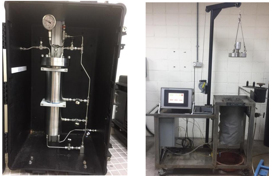
FIGURE 3.6. Pressure Vessel and Autoclave Machine Used for The Test
