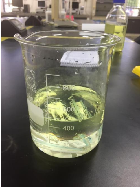
FIGURE 3.5. PVDF Samples in Hydrocarbon and Distilled Water Mixture
