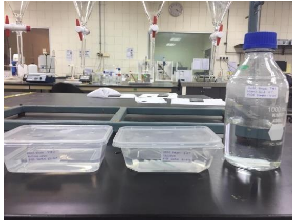
FIGURE 3.4. Samples Immersed in Distilled Water, Seawater and Nitric Acid
