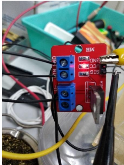
Figure 3.3: IRF520 MOSFET Driver Module
