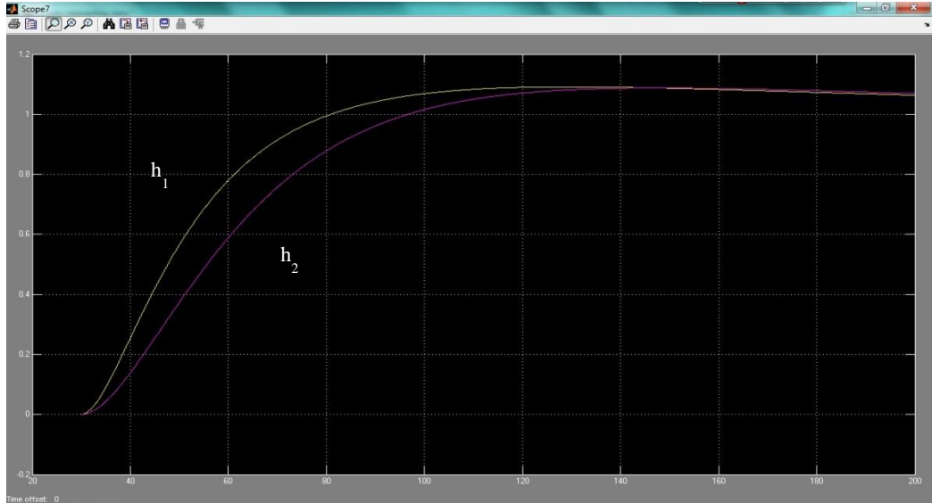
Figure 20 - Levels for PID Controller
