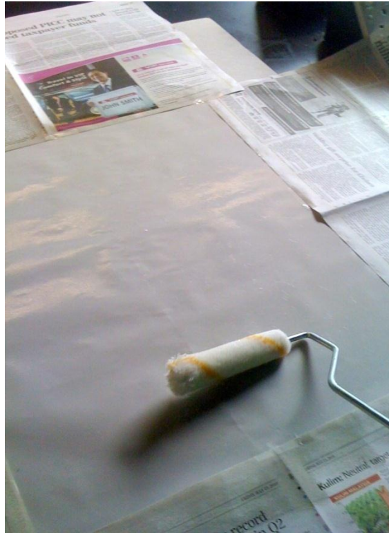
Figure 27 Mixture of silicon with thinner applied onto the tracing paper
