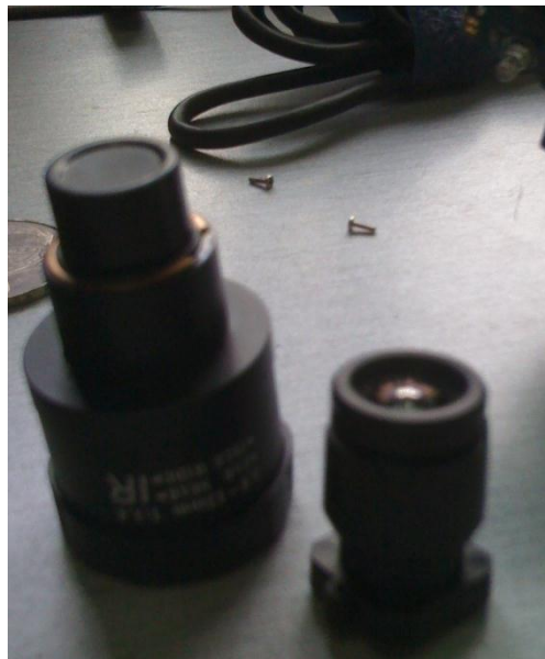
Figure 18 Varifocal lenses on the left side and standard lenses on the right side
