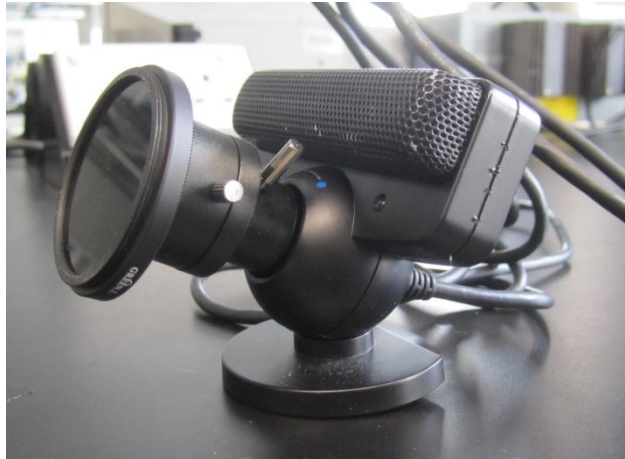
Figure 23 SONY PS3 Eye camera with IR filter and varifocal lens
