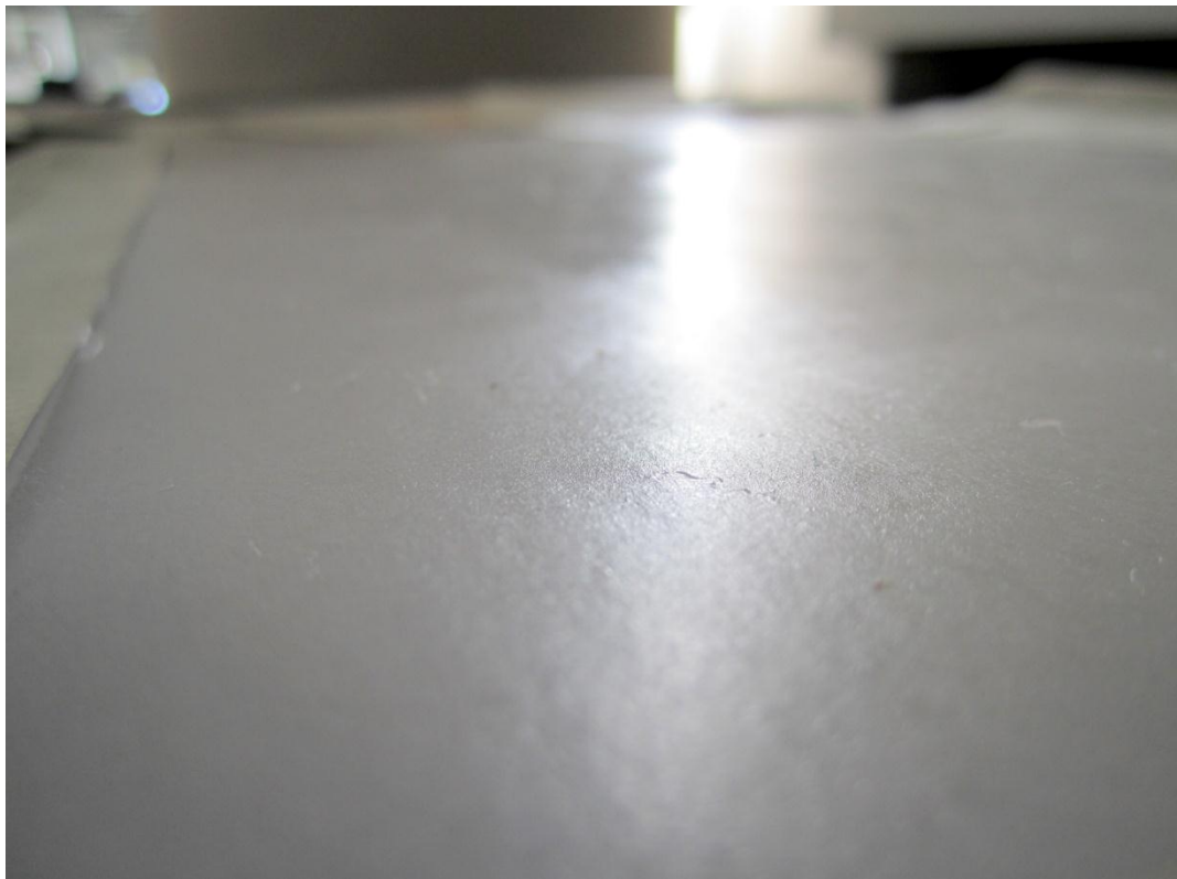
Figure 28 Smooth surface of the silicon and thinner mixture setup
