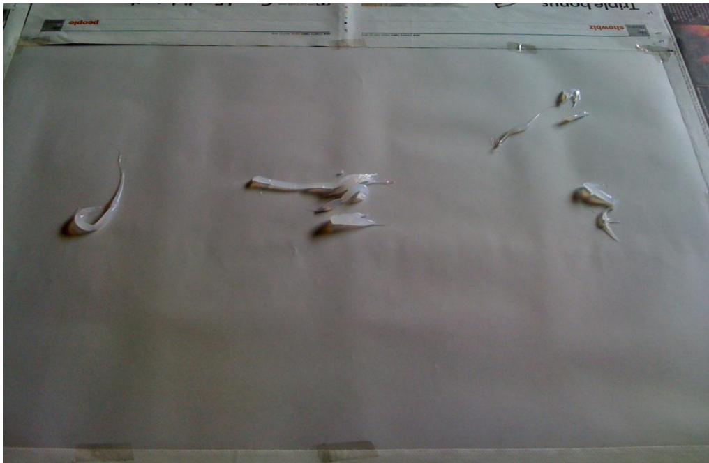
Figure 25 Silicon is applied directly onto tracing paper
