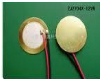
Figure 3: Piezoelectric Component
