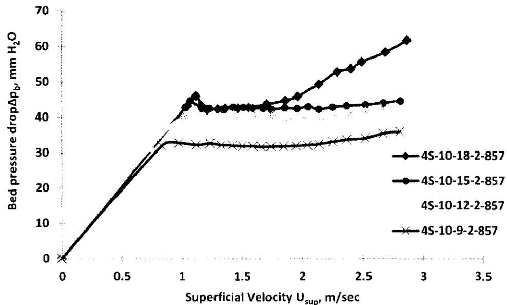
Figure 5.8: Bed pressure drop versus superficial velocity at various distributor blade overlap angles
