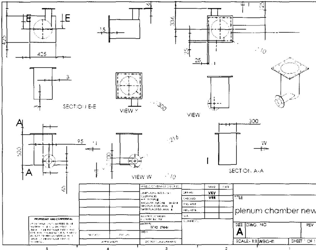
Figure 3.3: Plenum chamber design drawing
