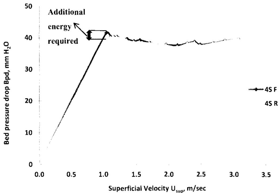
Figure 5.36: Plot demonstrating the hysteresis in 4 mm spherical type particle
