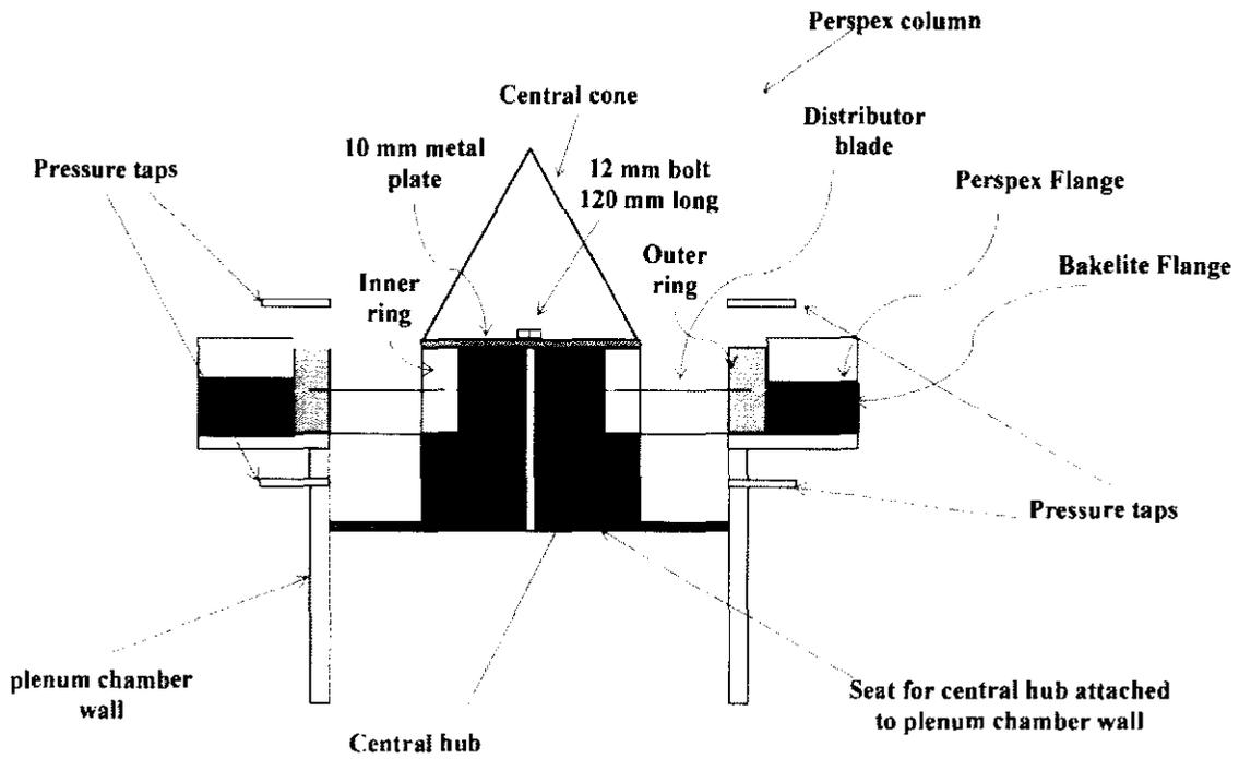
Figure 3.27: A cross sectional view of the SFB setup
