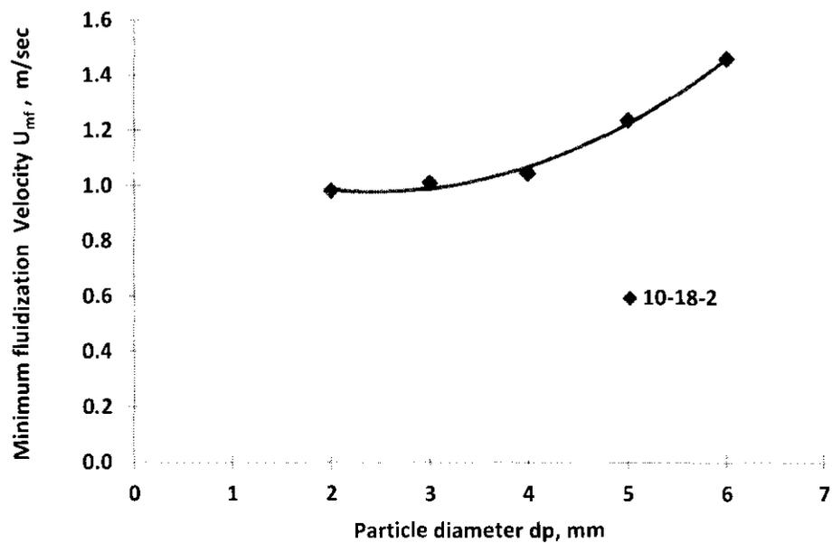
Figure 5.19: Minimum fluidizing velocity versus bed particle diameter
