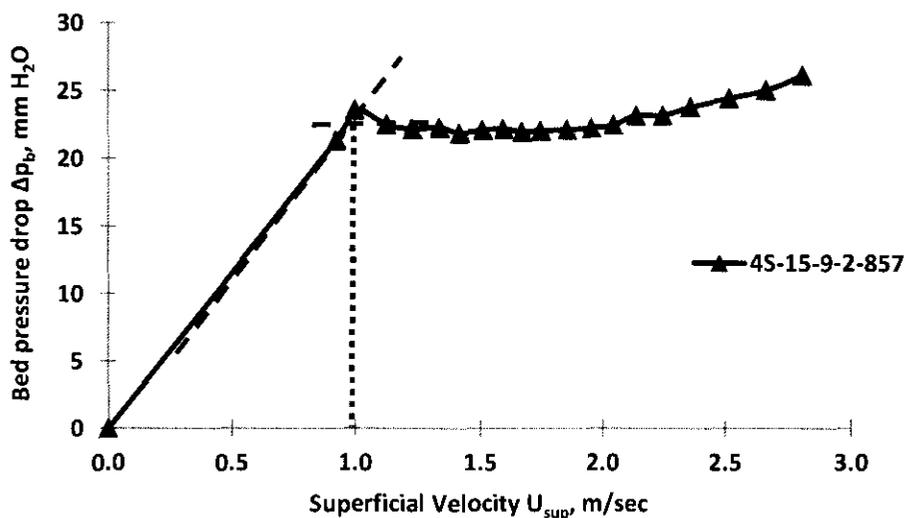
Figure 5.16: Bed pressure drop versus superficial velocity illustrating the method to find minimum fluidizing velocity,  $U_{mf}$
