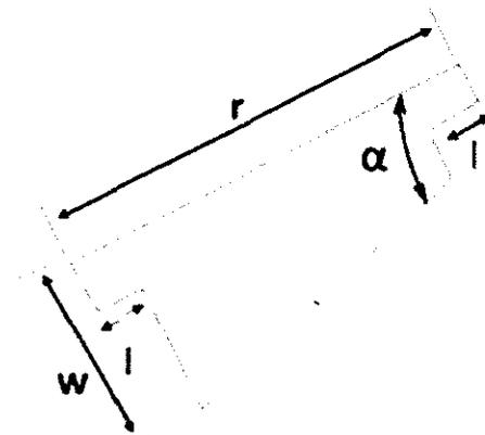
Figure 3.24: Trapezoidal shaped blade used in the work
