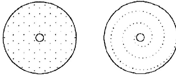
Figure 2.21: (a) Uniform pitch distributor (b) Spiral pitch distributor [31]
