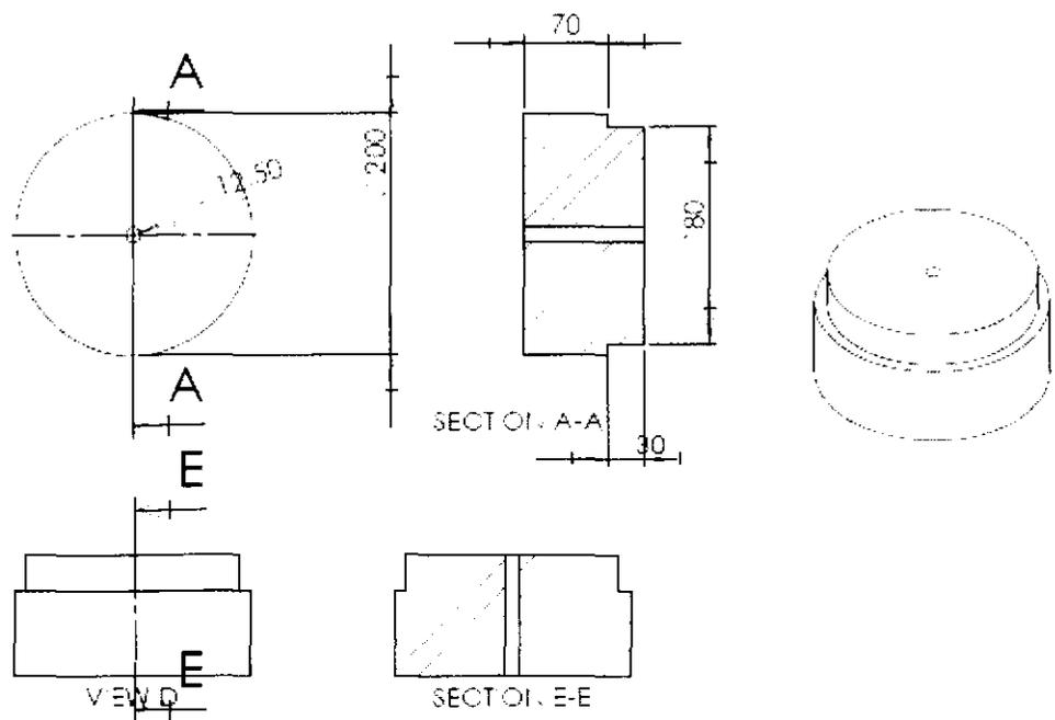
Figure 3.19: Design drawing of central hub of annular spiral distributor
