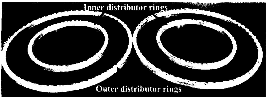
Figure 3.21: Outer and inner rings of annular spiral distributor realized
