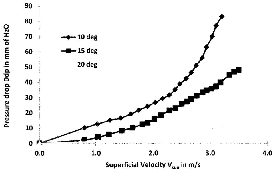
Figure 5.2: Distributor pressure drop versus superficial velocity at different blade inclinations
