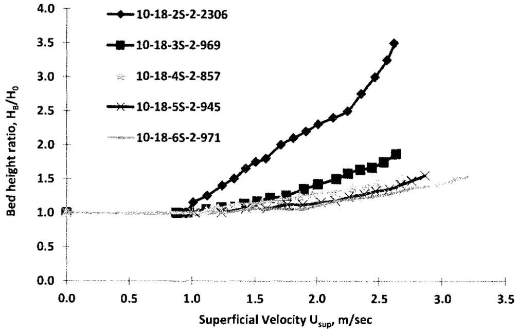
Figure 5.25: Bed height versus superficial velocity for different size particles
