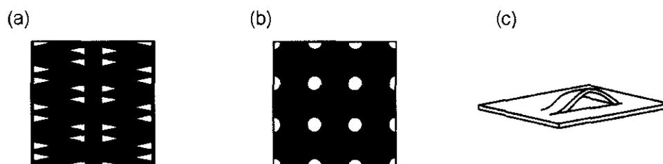
Figure 2.20: Details of distributor designs (a) Dutch weave mesh; (b) Perforated plate; (c) Punched plate [90]
