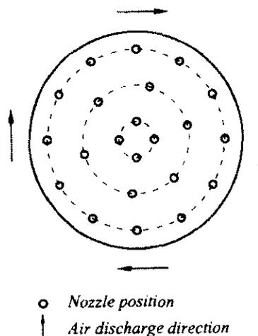
Figure 2.23: Illustration of the multi-horizontal nozzle distributor (top-view) [92]
