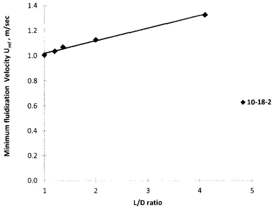
Figure 5.20: Minimum fluidizing velocity versus L/D ratio for particles of various shapes
