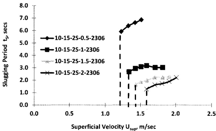
Figure 5.30: Plot of slugging time versus superficial velocity for various bed weights
