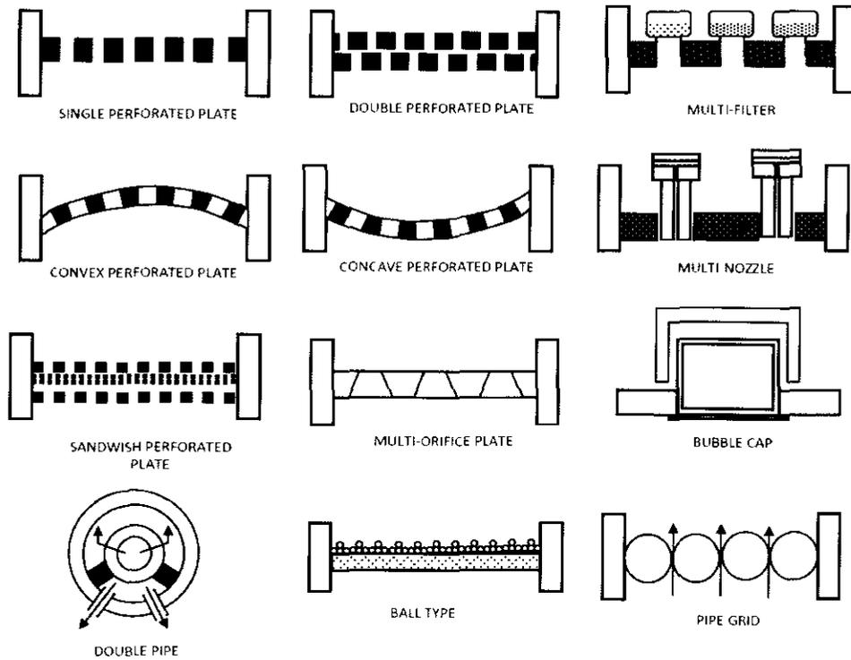
Figure 2.18: Examples of distributors in common use [44].
