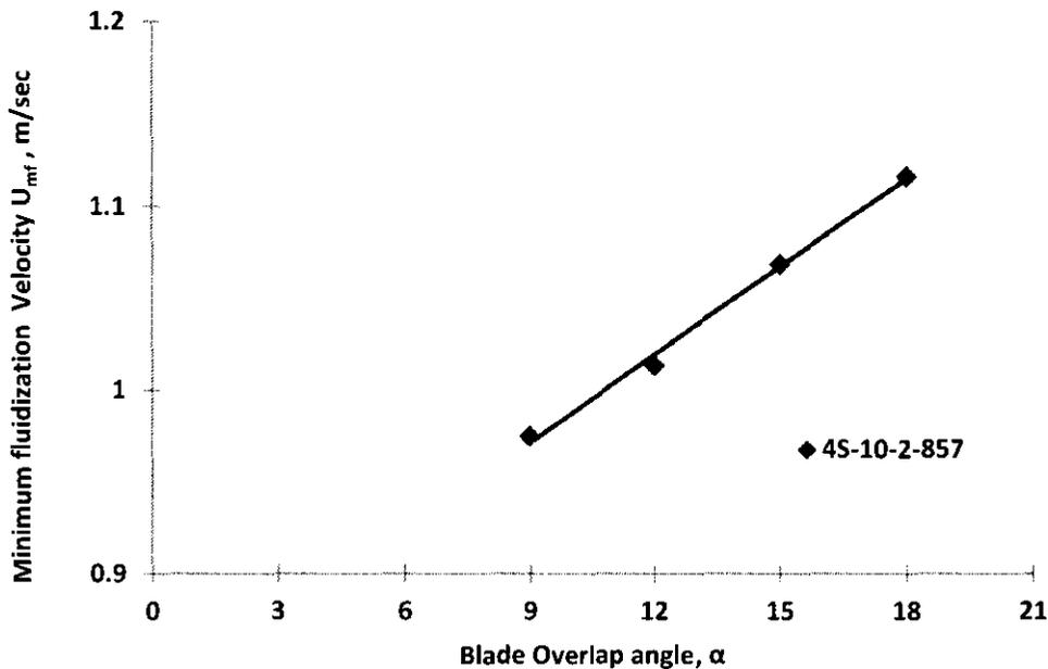
Figure 5.18: Minimum fluidizing velocity versus blade overlap angle
