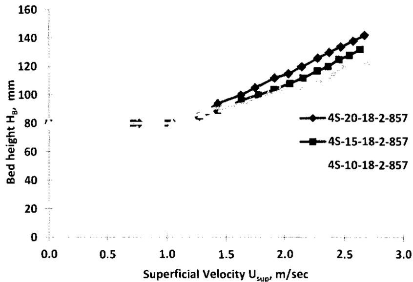
Figure 5.23: Bed height versus superficial velocity for different blade inclination angles
