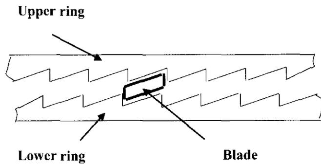
Figure 3.20: Section view describing assembly of blades and distributor rings
