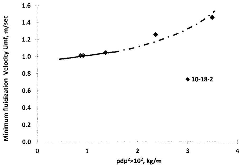
Figure 5.22: Minimum fluidizing velocity versus  $f(\rho d_p)$
