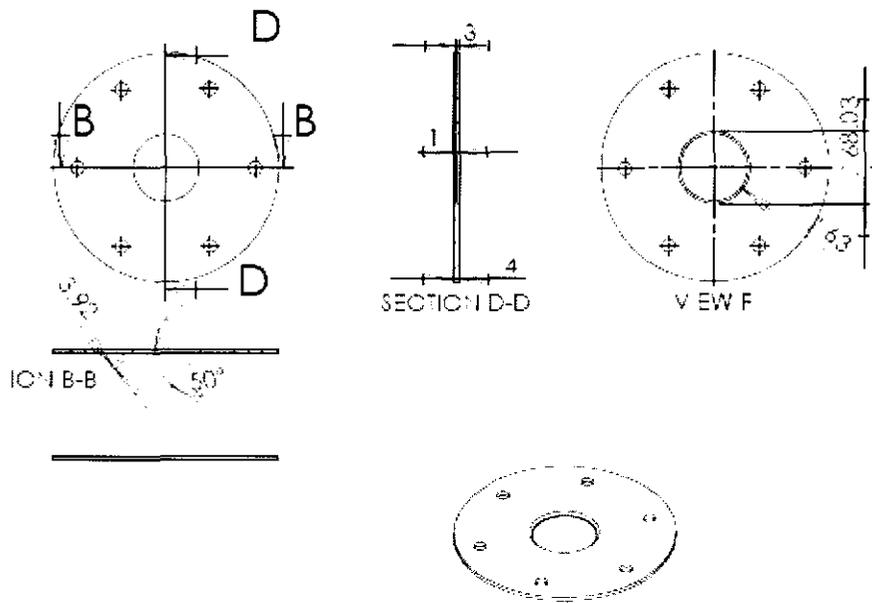
Figure 3.7: Design drawing of high flow orifice plate
