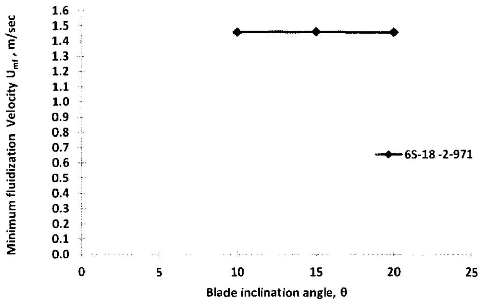
Figure 5.17: Minimum fluidizing velocity versus blade inclination angle
