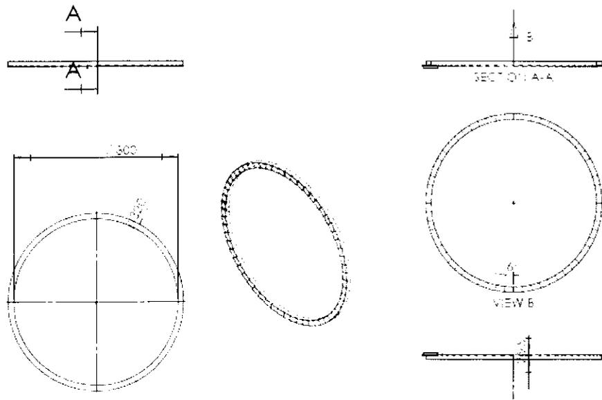
Figure 3.16: Design drawing of outer ring of annular spiral distributor
