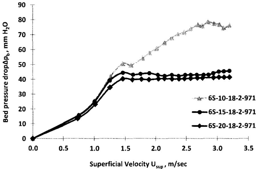
Figure 5.7: Bed pressure drop versus superficial velocity at various distributor blade inclination angles
