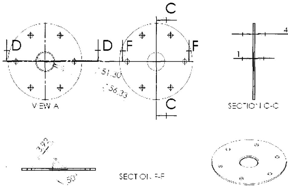
Figure 3.8: Design drawing of low flow orifice plate
