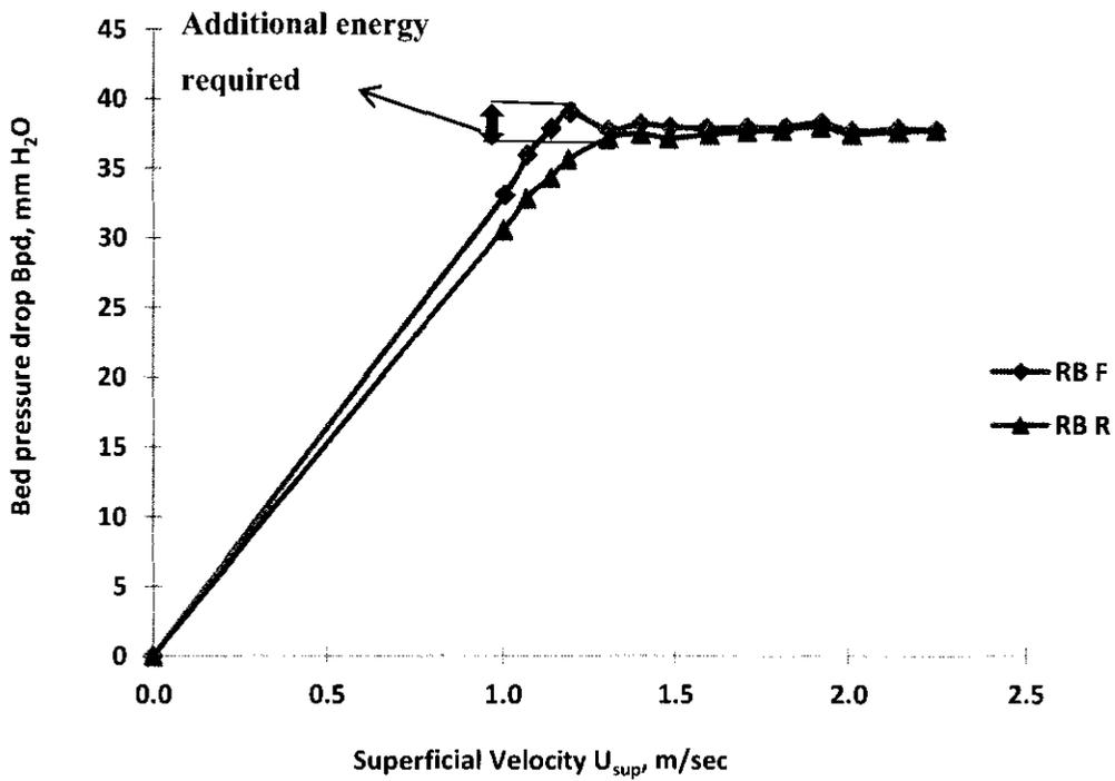
Figure 5.38: Plot demonstrating the hysteresis in rice bead type particles
