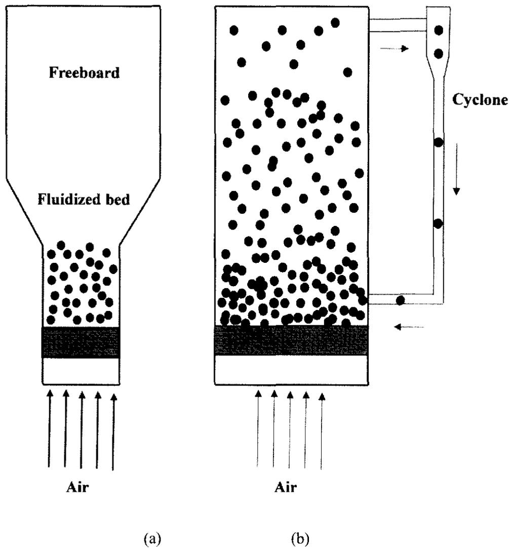
Figure 2.2: Schematic of (a) bubbling and (b) circulating fluidized bed [10]
