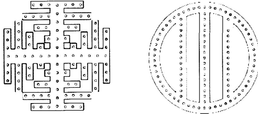
Figure 2.25: Branched pipe distributor and circular pipe distributor [92]
