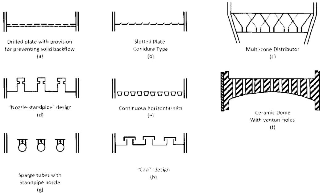
Figure 2.17: Examples of distributors in common use [44]
