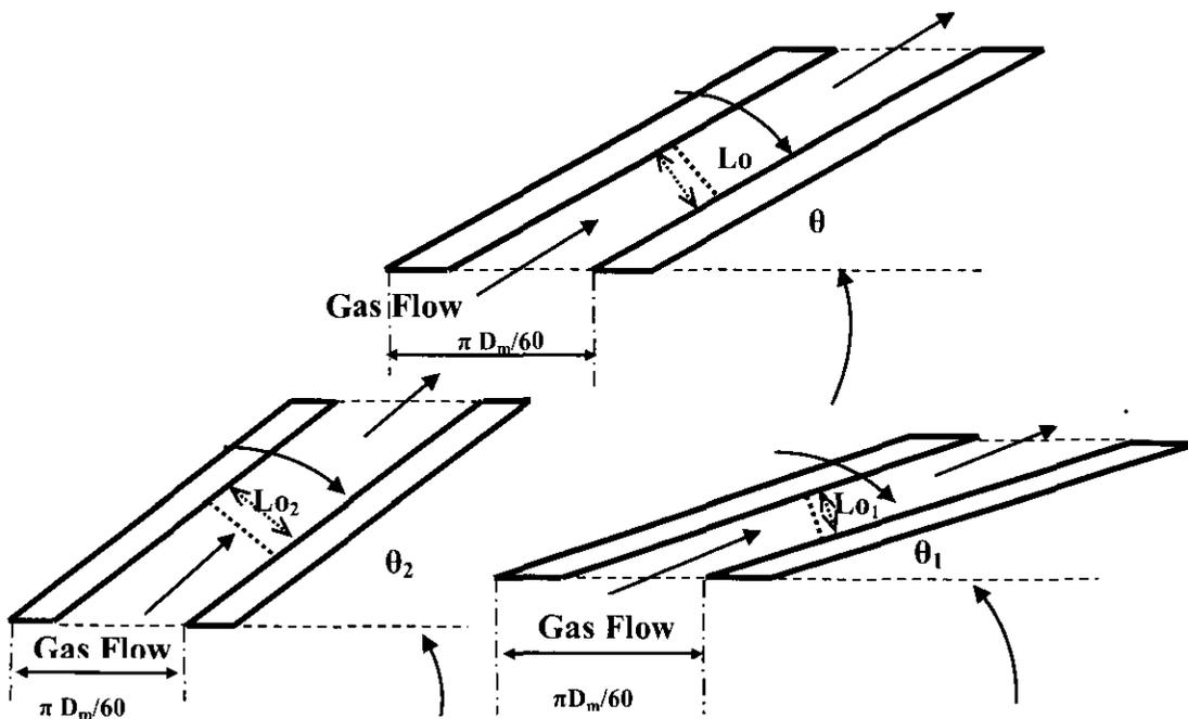
Figure 5.3: Illustration of blade inclination angle and blade opening
