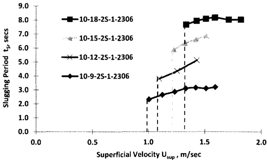
Figure 5.32: Plot of slugging time versus superficial velocity for different blade overlap angles
