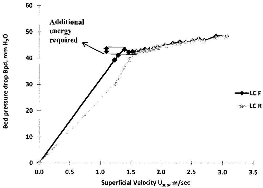
Figure 5.37: Plot of demonstrating the hysteresis in cylindrical type particles
