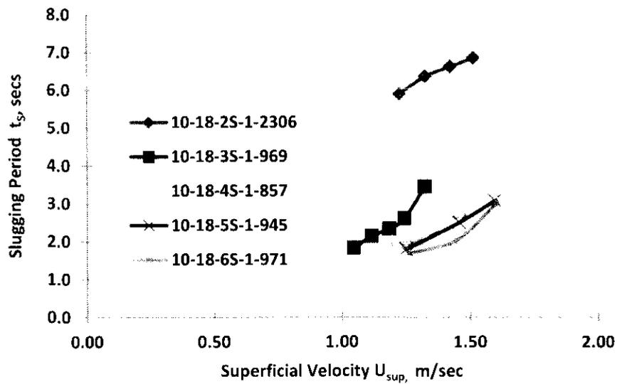
Figure 5.34: Slugging time versus superficial velocity for different particle sizes
