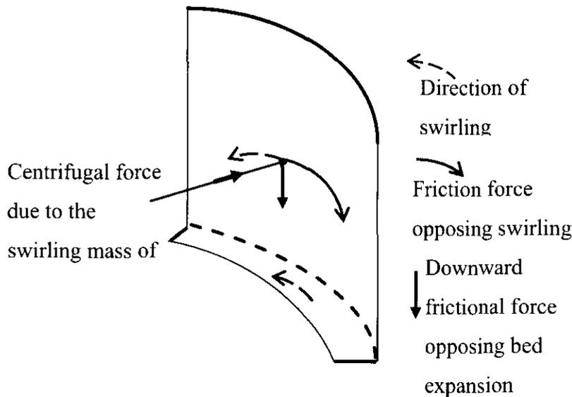
Figure 5.1: Free body diagram of forces acting on the swirling fluidized bed
