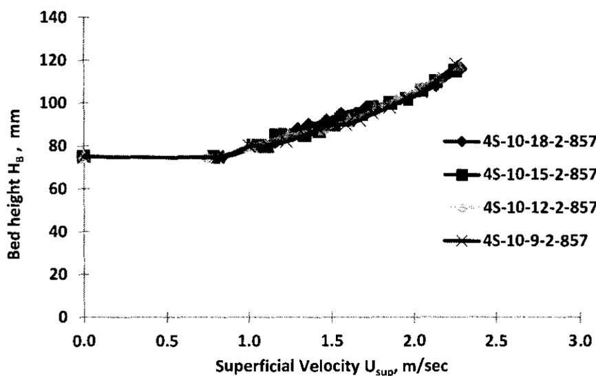
Figure 5.24: Bed height versus superficial velocity for different angles of overlap
