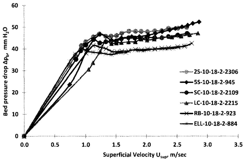
Figure 5.15: Bed pressure drop versus superficial velocity for particles with different densities
