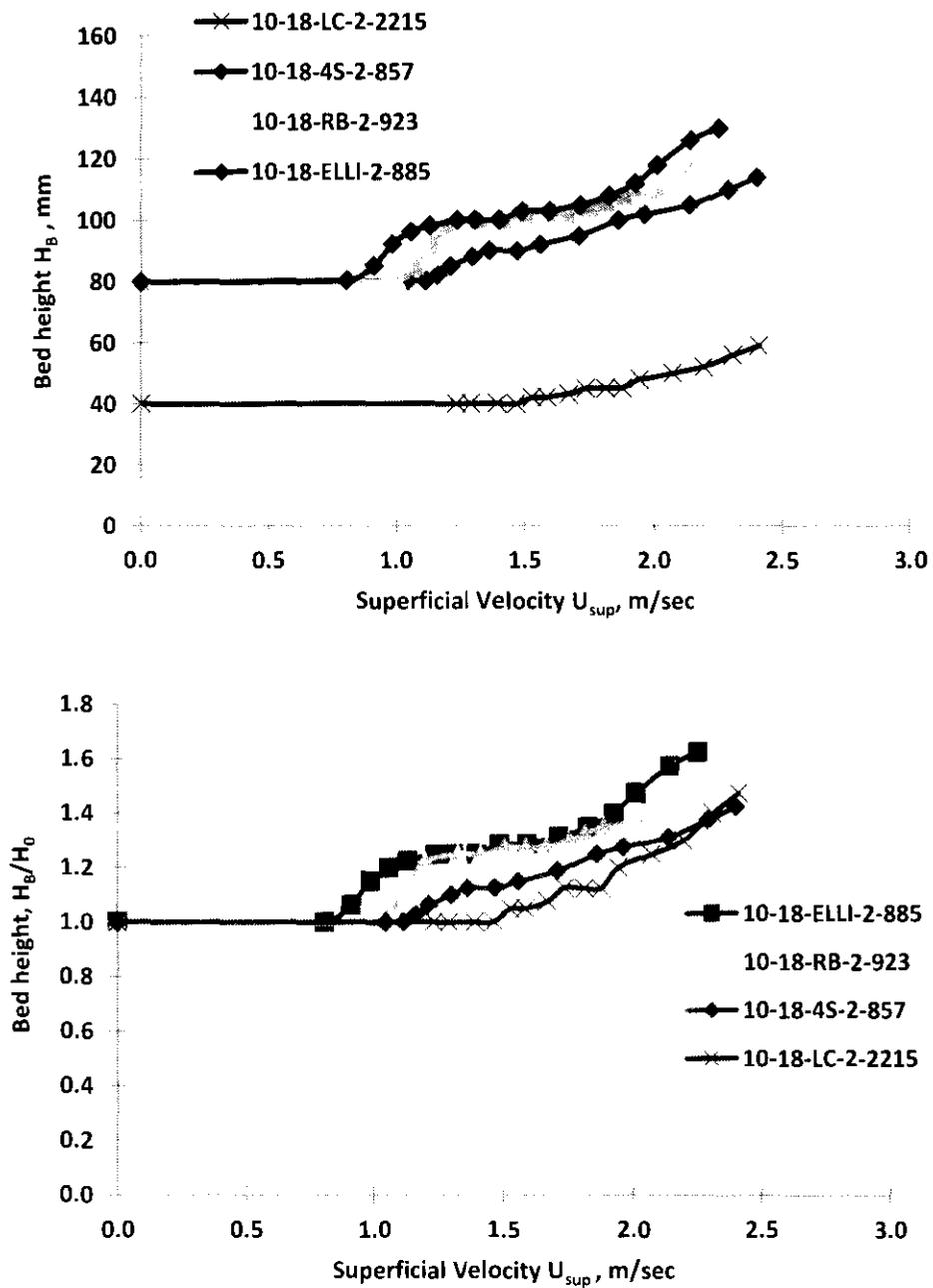
Figure 5.26: Bed height versus superficial velocity for particles of different shape
