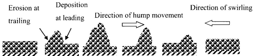
Figure 5.28: Different stages of the bed in a slug-wave regime
