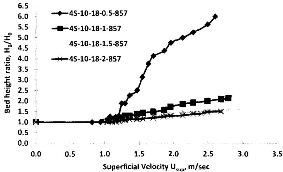
Figure 5.27: Bed height versus superficial velocity for different bed weights
