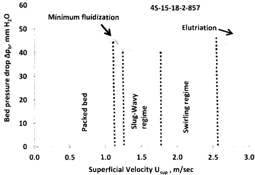
Figure 5.6: Plot of bed pressure drop versus superficial velocity
