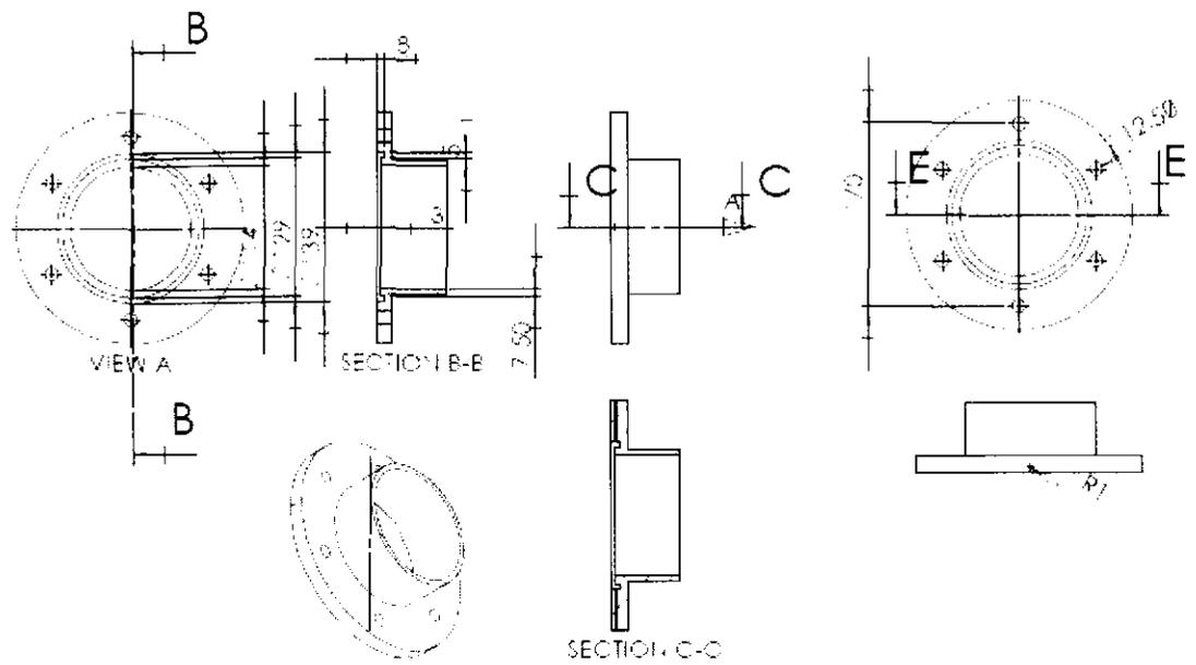
Figure 3.9: Design drawing of flanges for orifice meter
