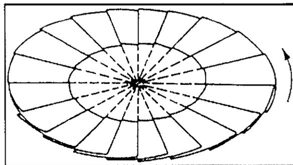
Figure 2.13: The annular spiral distributor as used by Sreenivasan and Raghavan.
