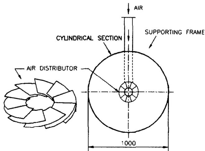
Figure 2.10: Design details of air supply of the experimental rig with annular-spiral air distributor as used by Kaewklum *et al.* [37]
