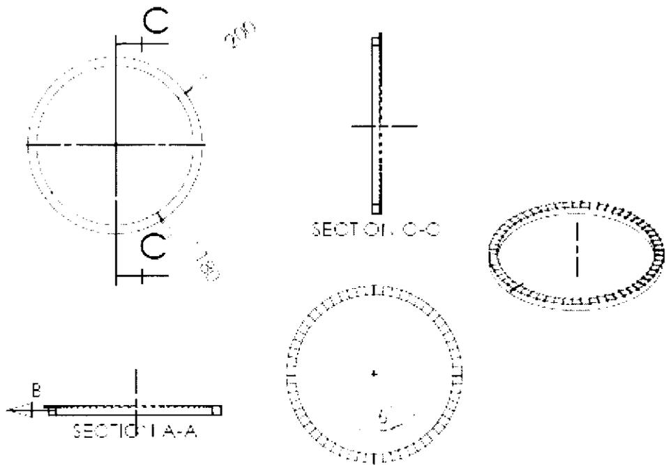
Figure 3.17: Design drawing of inner ring of annular spiral distributor
