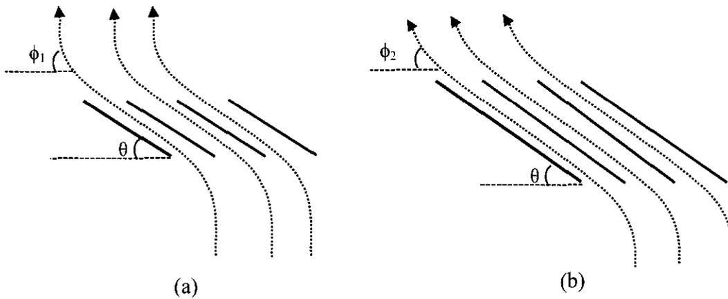
Figure 5.9: Fluidizing gas direction after passing through the distributor of variable overlap angles (a) shorter overlap (b) longer overlap
