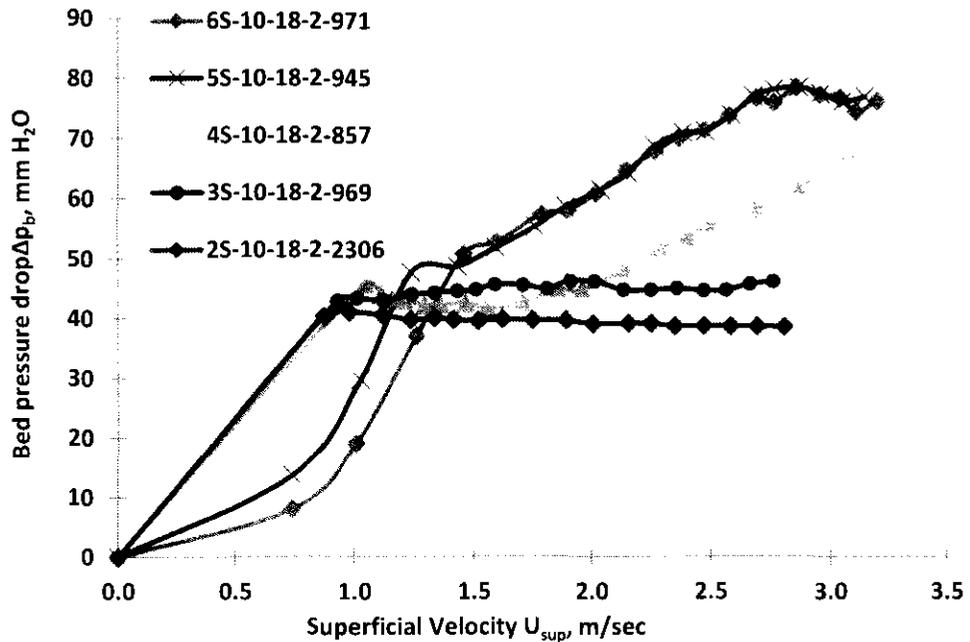
Figure 5.10: Bed pressure drop versus superficial velocity for various sizes of spherical bed particles
