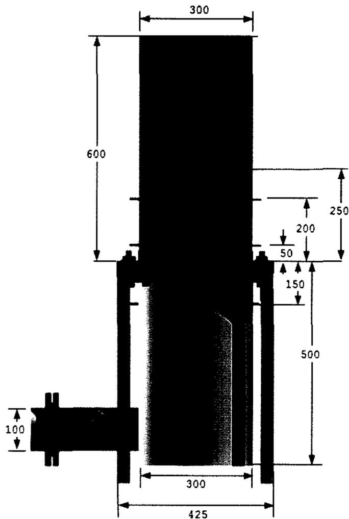
Figure 2.14: Schematic of the experimental set-up used by Sreenivasan and Raghavan [39].
