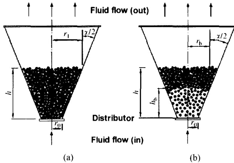
Figure 2.16: Sand conical beds in (a) fixed and (b) partially fluidized state [82].
