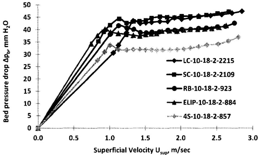
Figure 5.13: Bed pressure drop versus superficial velocity
