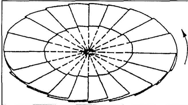
Figure 3.14: The annular spiral distributor as used by Sreenivasan and Raghavan [39]
