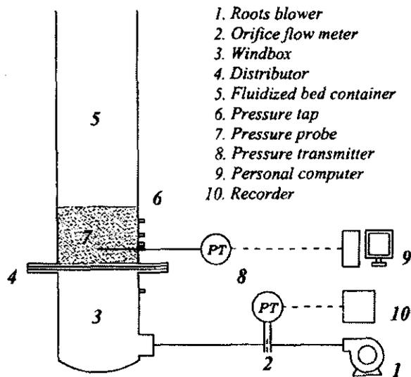
Figure 2.24: A Schematic diagram of the fluidized-bed [92]
