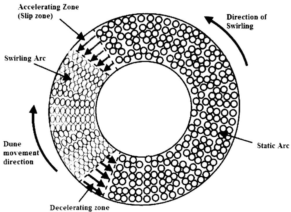
Figure 5.29: Top view of a swirling fluidized bed experiencing slug-wave
