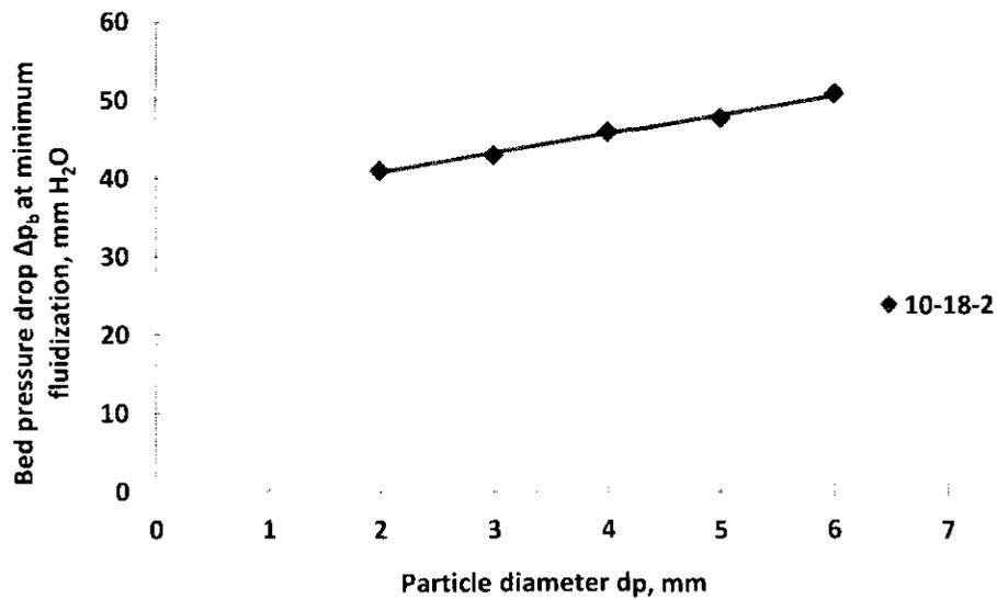
Figure 5.11: Bed pressure drop at minimum fluidization versus particle diameter
