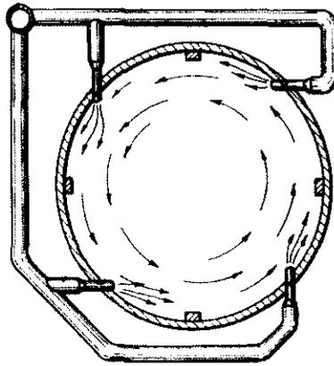
In another variant of the fluidized bed, as in Figure 2.3, a swirl is imparted to the fluidized bed by injecting secondary air tangentially into the freeboard. This is a concept brought forth and patented by Sowards [29], which the author refers to as the vortexing fluidized bed (VFB), and uses a perforated plate as the air distributor.
