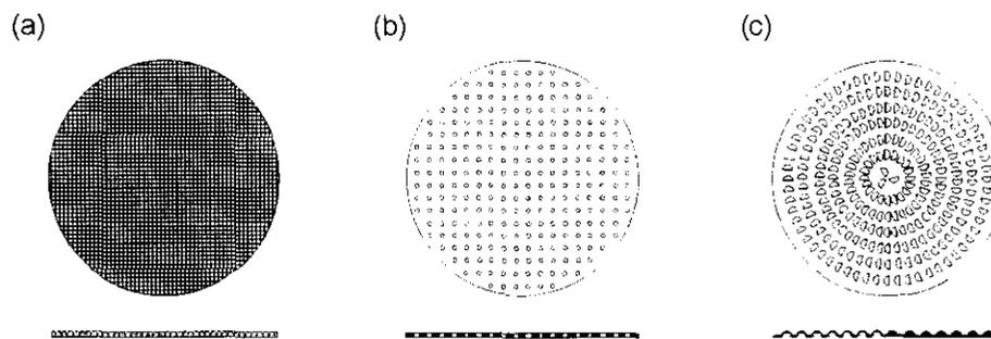
Figure 2.19: Distributor designs (a) Dutch weave mesh; (b) Perforated plate; (c) Punched plate [90]
