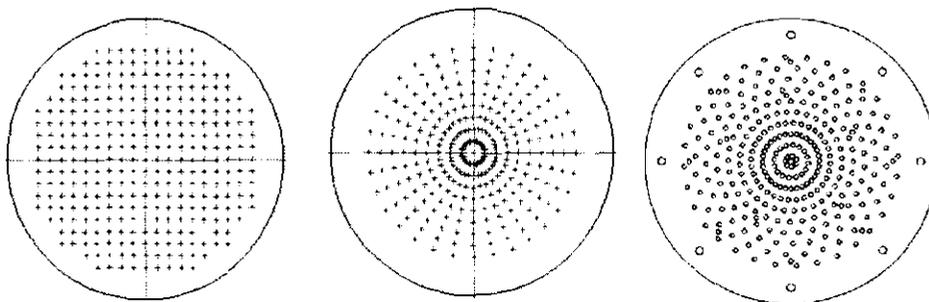
Figure 2.22: Distributor design, (a) square pitch distributor (SPD), (b) circular pitch distributor (CPD) and (c) semi-circular pitch distributor (SCPD) [91]
