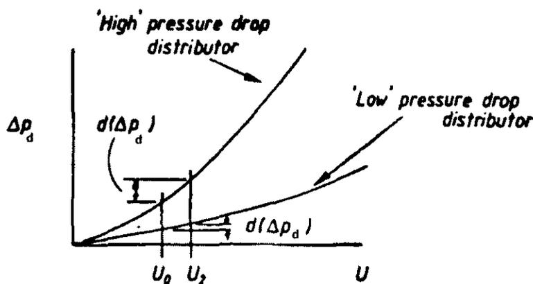
Figure 2.15: High and low pressure drop distributors [52]
