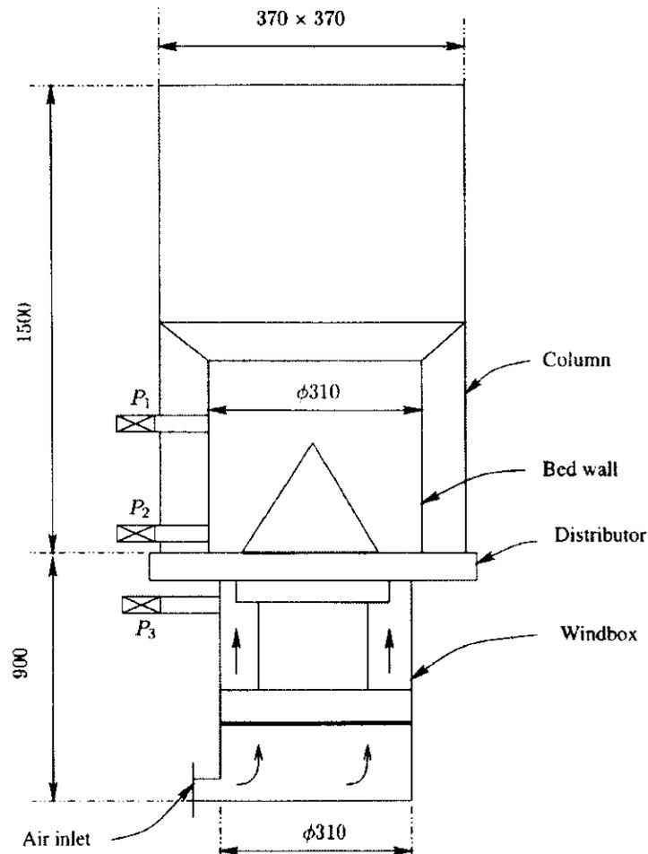
Figure 4.4: Sketch of swirling fluidised bed showing location of pressure taps
