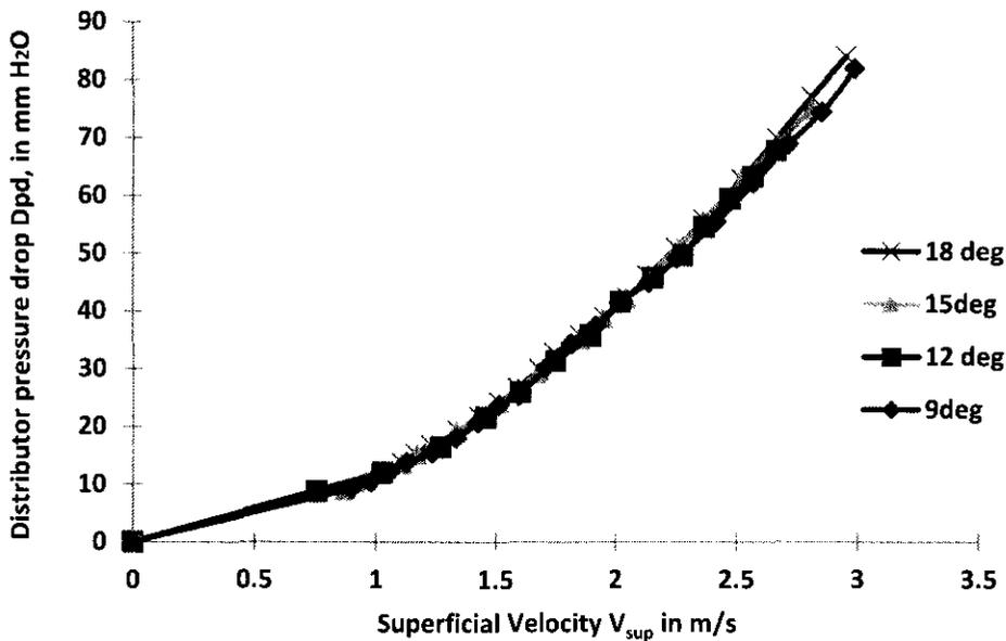
Figure 5.5: Distributor pressure drop versus superficial velocity at different blade overlap angles
