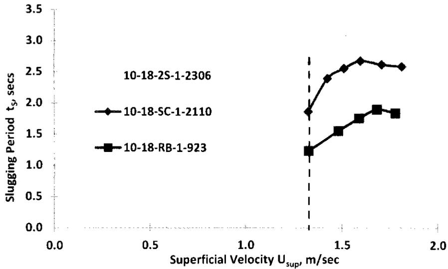
Figure 5.31: Plot of slugging time versus superficial velocity for different shapes of particles
