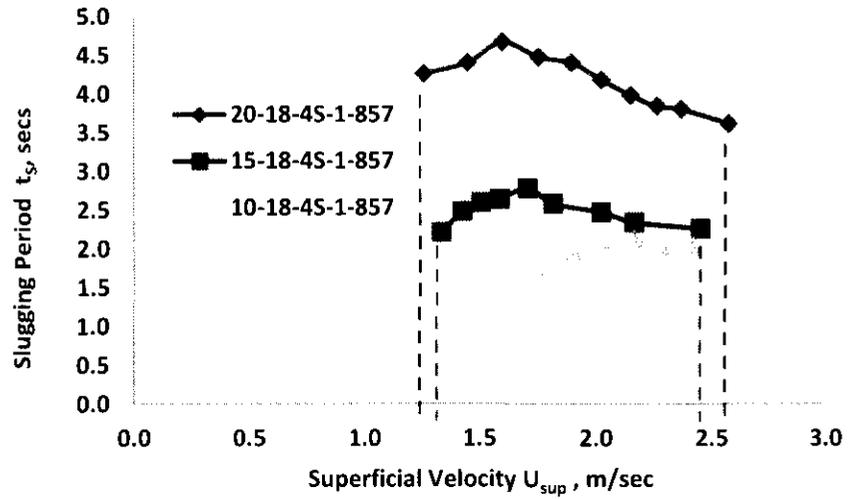
Figure 5.33: Plot of slugging time versus superficial velocity for different blade inclinations
