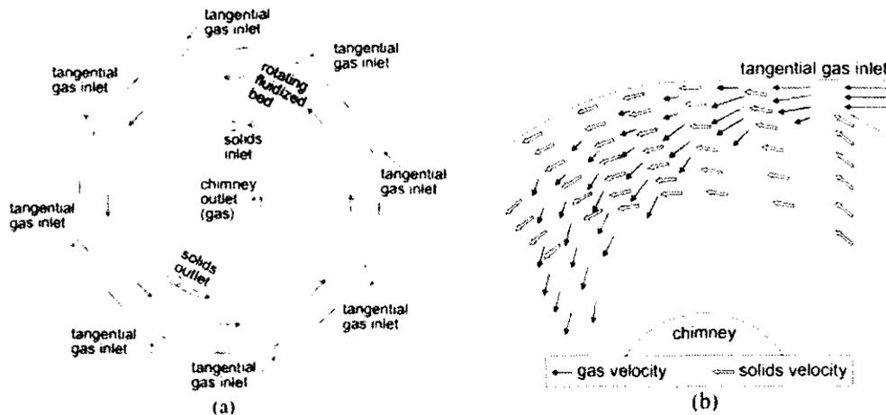
Figure 2.5:(a) 2-D section of the fluidizing chamber; (b) Behavior of the gas and particle velocities near the tangential gas inlet of the fluidizing chamber [32]
