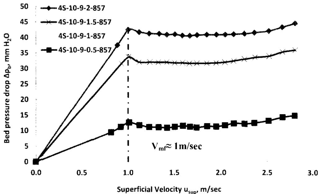
Figure 5.14: Bed pressure drop versus superficial velocity for various bed weights
