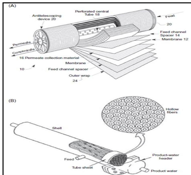
Figure 2.3: A typical spiral-wound flat-sheet membrane element (A) and hollow-fiber membrane module (B) (Cutaway sight of) [Source: (Han et al., 2018)].
