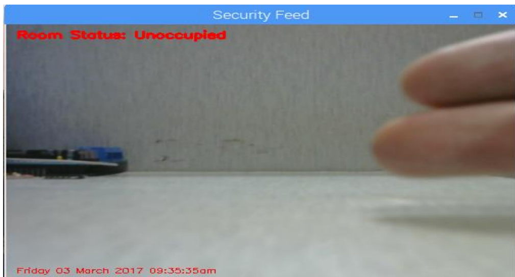
Figure 4.2: Room status unoccupied even with motion
