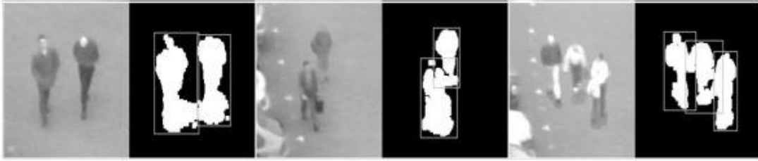
Figure 2: An object tracking based on research [14].
