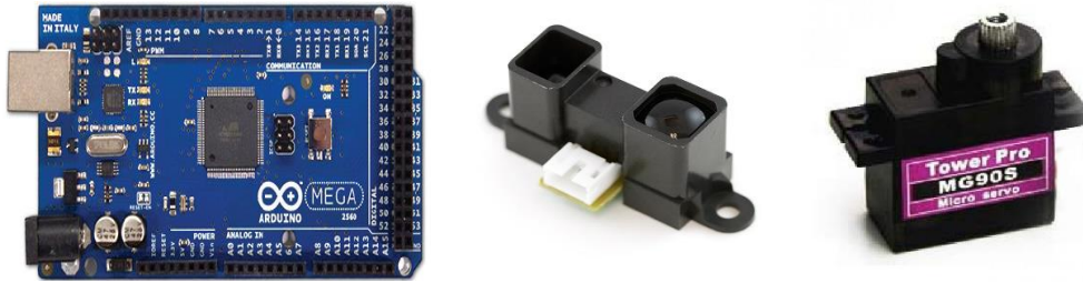
Figure 6 : Hardware Used for the Project (Arduino Mega, Sharp GP2Y0A02YK0F Infrared Sensor and Servo Motor)[2]
