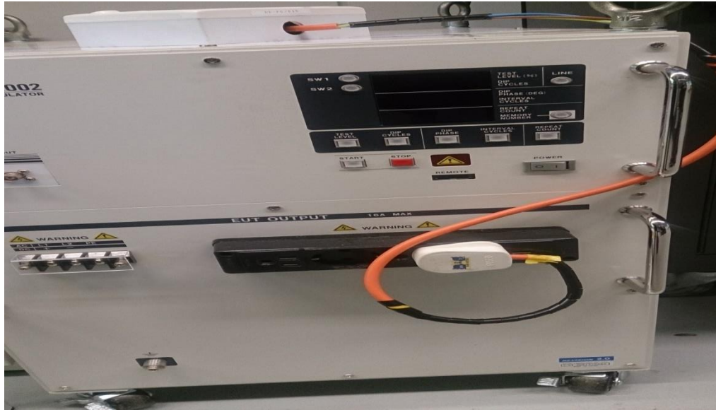
Figure 9: Single-phase voltage dip generator
