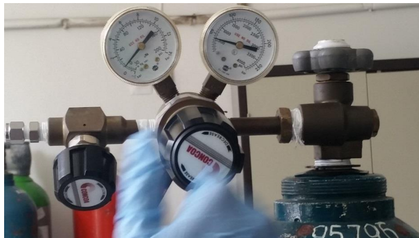
Figure 10: Flow control of oxygen.
