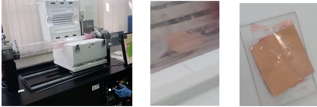
Figure 13: cooper foil insert into CVD machine and Graphene growth on copper foil
