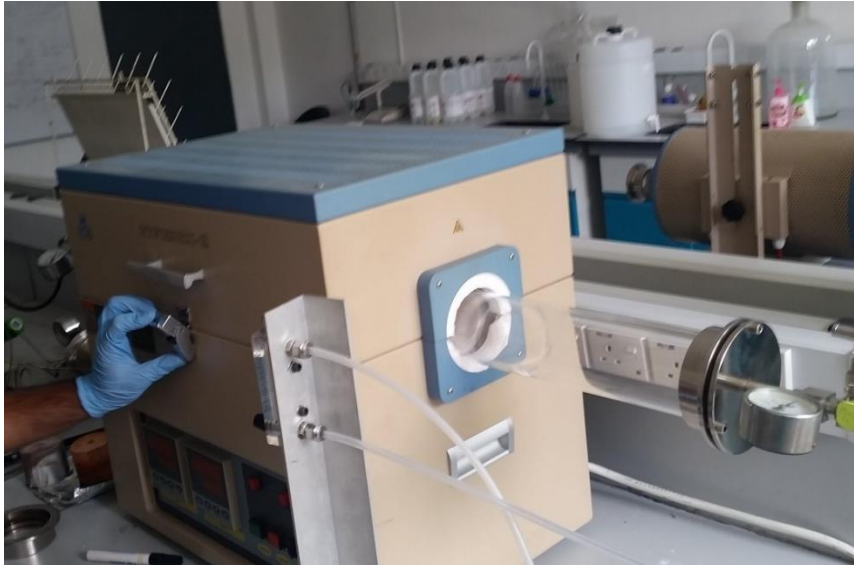
Figure 9: Reaction Chamber to growth silicon dioxide
