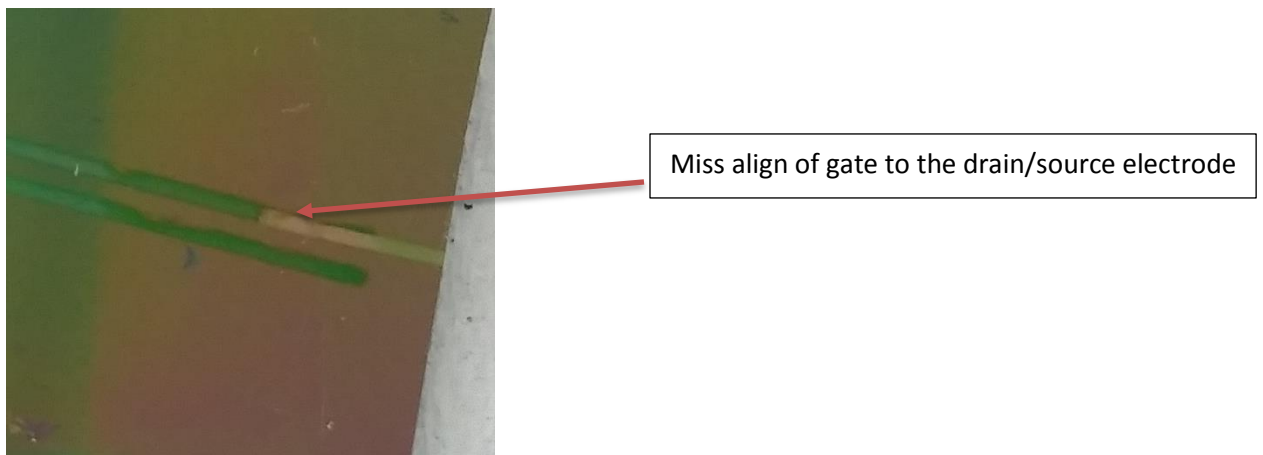
Figure 32: miss align electrode
