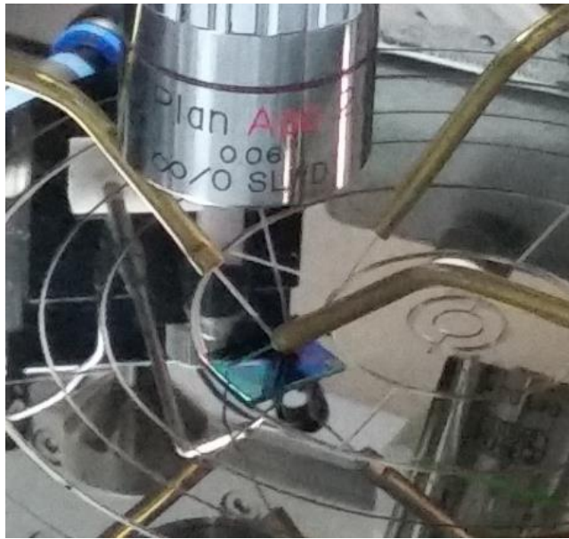
Figure 28: Measuring G-FET characteristic used Agilent B1500A
