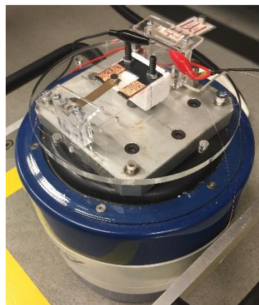
Figure 4.8: Hybrid Energy Harvester on Vibration Shaker
