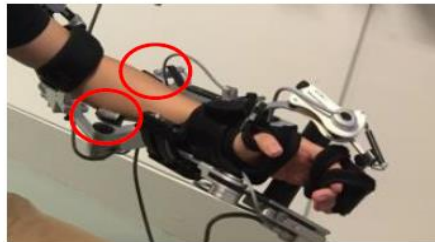
Figure 16: Obtaining the EMG signal utilizing the rehabilitation robotic.
