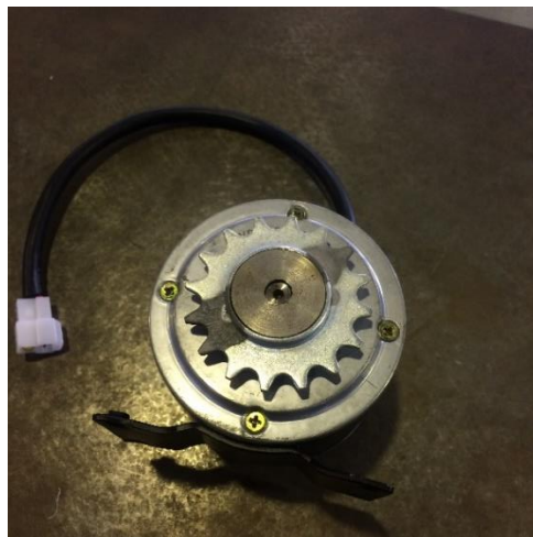
Figure 3.5: Custom-made sprocket installed on the motor
