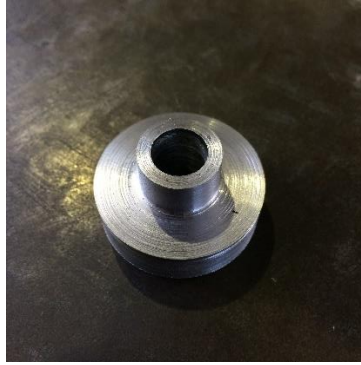
Figure 3.4: Lathing and parting process outcome
