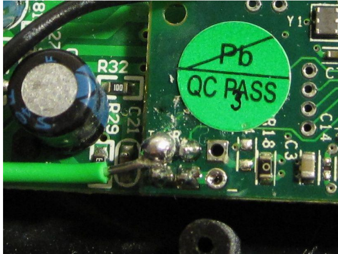
FIGURE 9: T pin soldered which will then be connected to the Arduino's RX port
