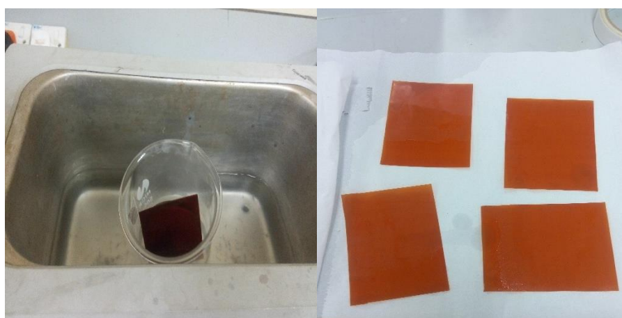
Figure 10: (a) Ultrasonication of polyimide film in acetone, (b) Cleaned polyimide film is then dried in room temperature.
