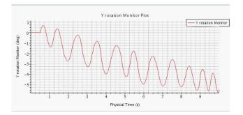
Figure 4. 4 Numerical Expected Yaw Motion with rotating fan blade
