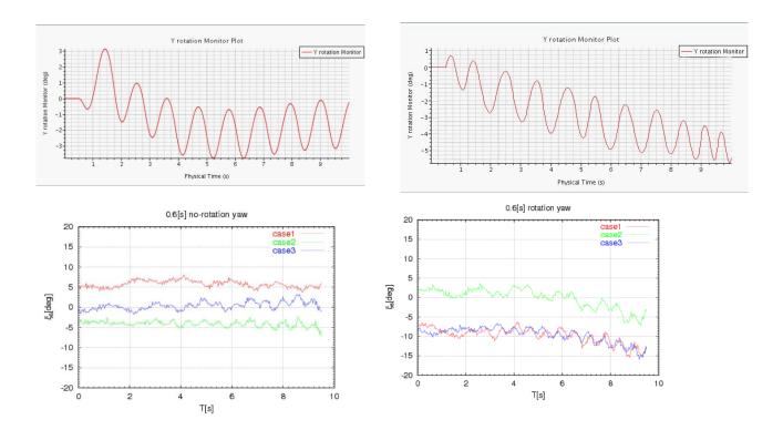
Figure 4. 5 Yaw Motion without and with rotating fan blade
