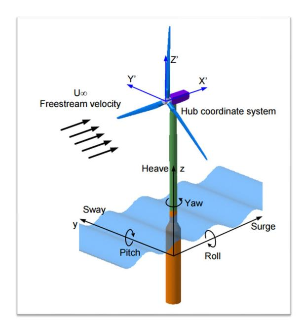
Figure 2. 1 Resultant motion produce in FOWT
