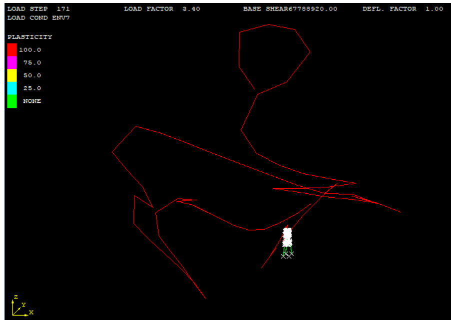
FIGURE 4.8 Platform EF Failure Condition in Collapse Output
