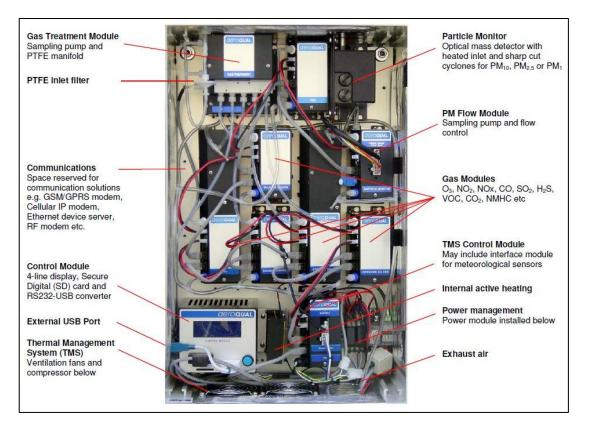
Figure 11: Aeroqual AQM 60 Station enclosed components.
