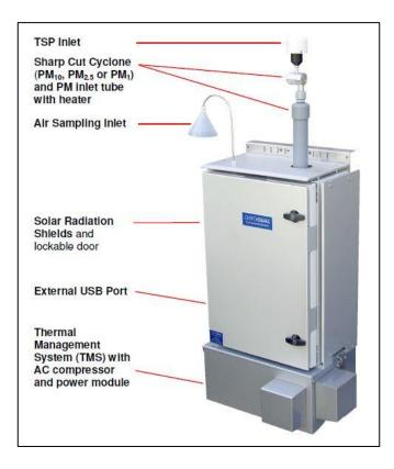
Figure 10: Aeroqual AQM 60 Station external components
