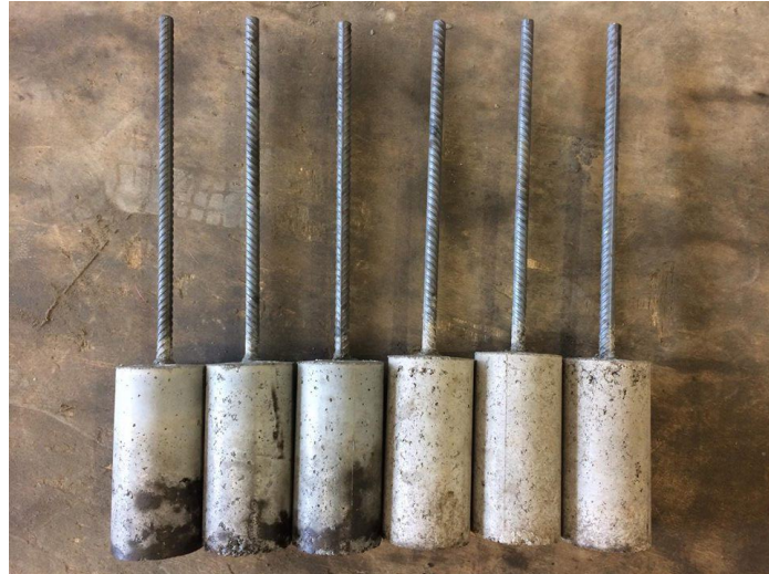
Figure 3.24: The specimen for pull-out test
