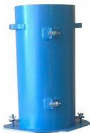
Figure 3.11: Concrete cylindrical mould
