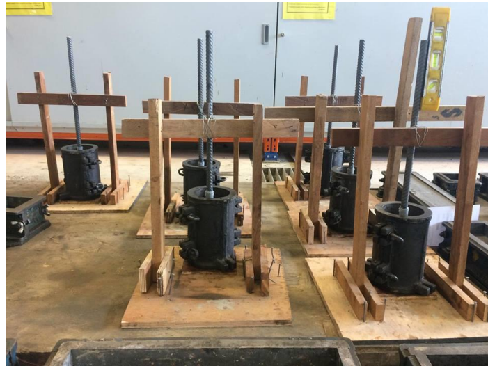
Figure 3.22: Mould for pullout test
