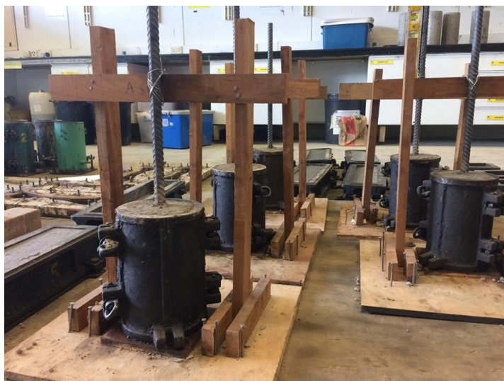
Figure 3.23: Concreting for pullout test
