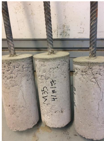
Figure 4.5: Sample after pull-out test
