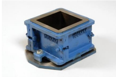
Figure 3.10: Concrete cube mould
