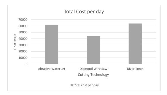
Figure 10 Total Cost of Cutting Technology per day
