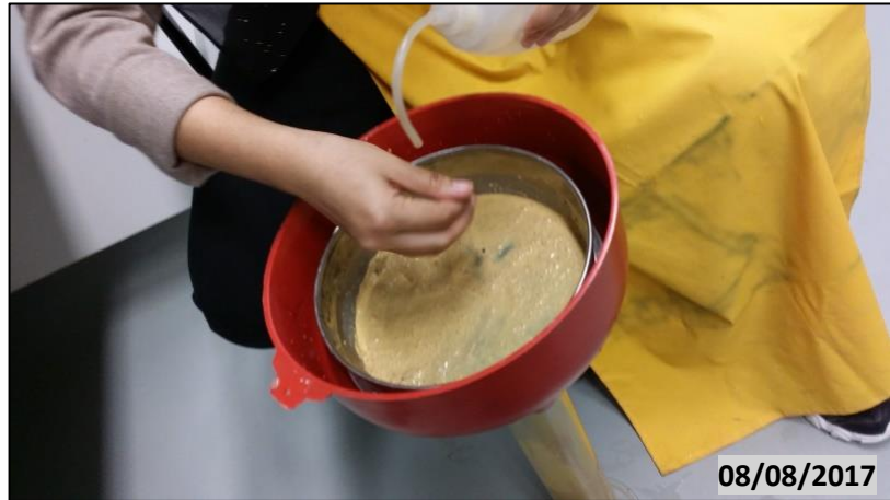
Figure 3-11: Preparation for hydrometer test by wet sieving (Source: Author)
