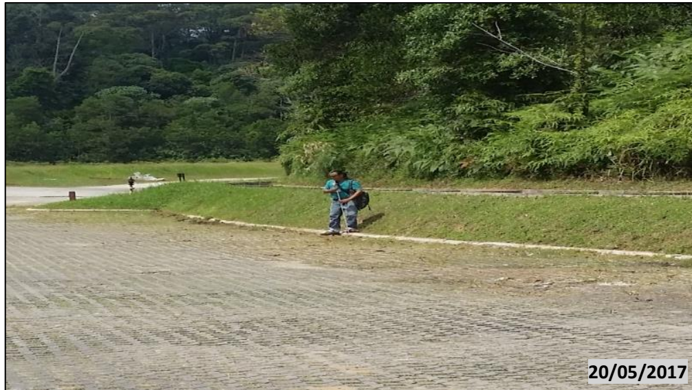
Figure 3- 3: Holding Prism Pole for Data Collection (Source: Author)
