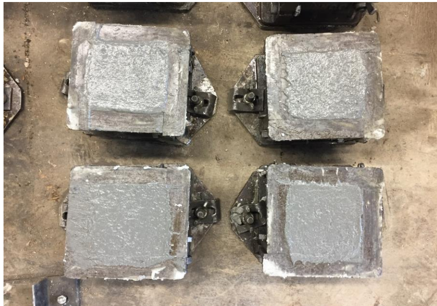
Figure 7 Concrete moulds cube size
