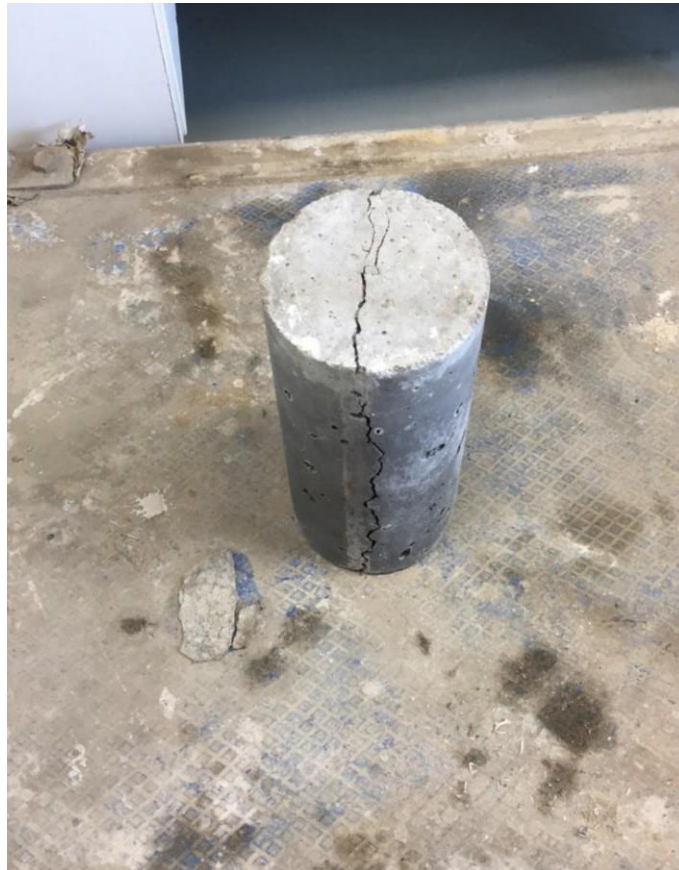
Figure 19 The Vertical Crack on Sample
