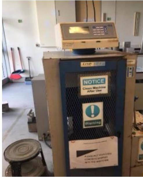
Figure 9 Compressive Strength Machine
