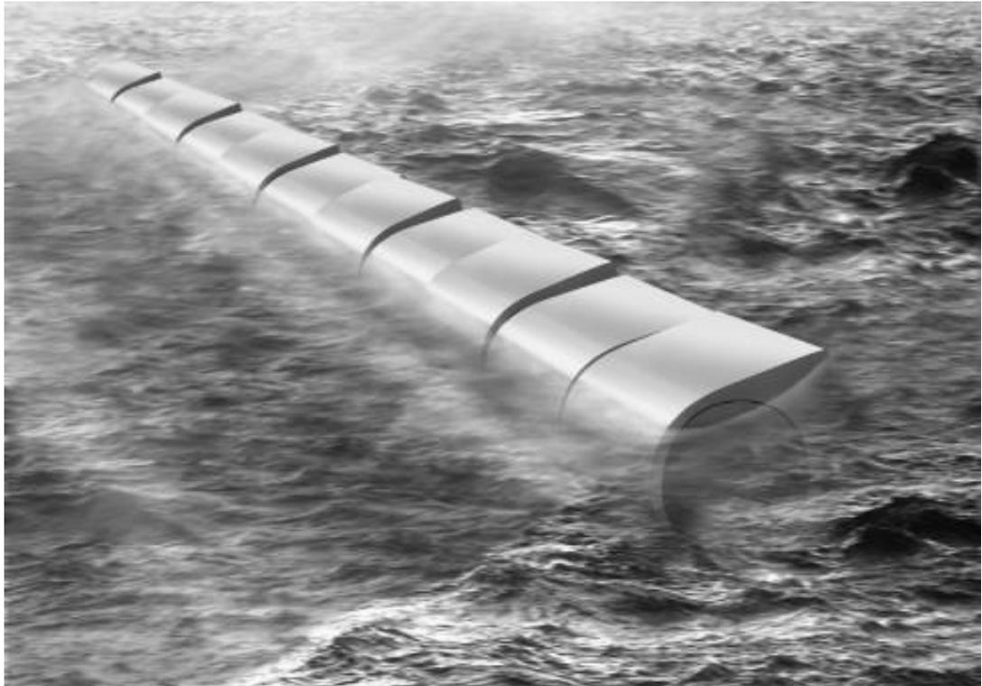
FIGURE 2.6: Salter's Nodding Duck wave energy converter.
