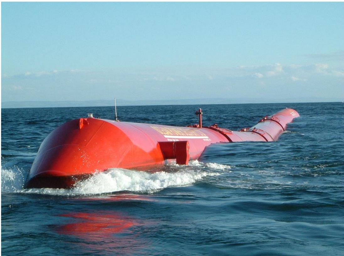
FIGURE 2.4: Pelamis wave energy converter in open sea.
