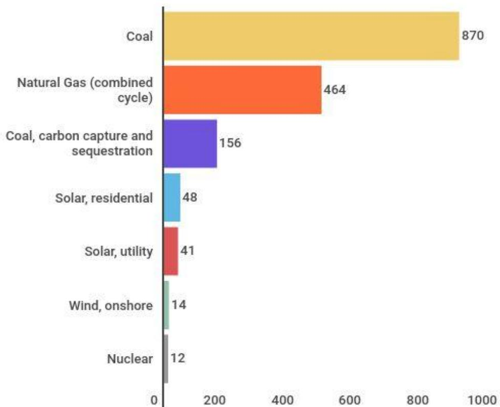
grams of CO2 per kilowatt of electricity produced
