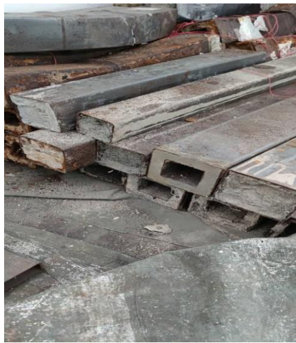
Figure 6 shows the Steel Tube Beams that will be used for the testing
