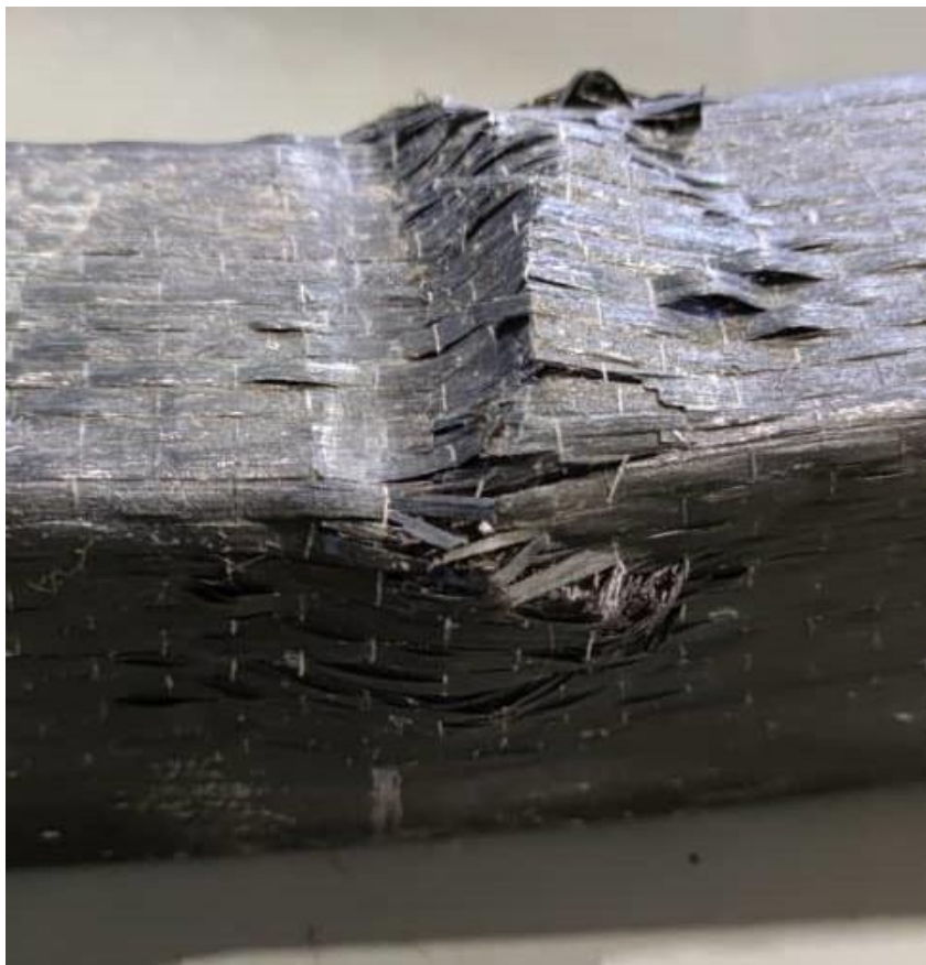
Figure 13 shows the CFRP rupture on CFST-3L
