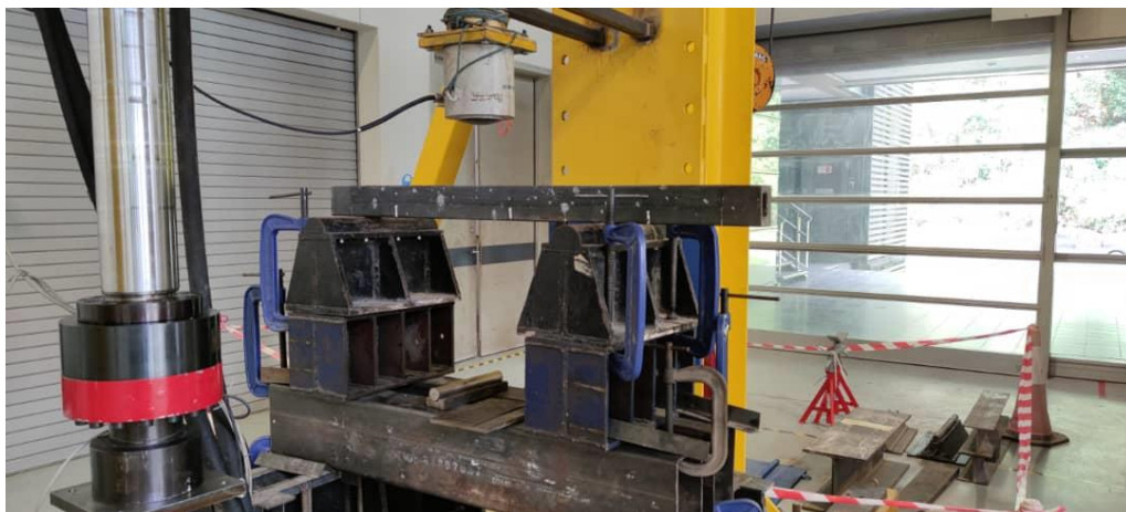
Figure 8 shows the set up for the testing of CFST wrapped with CFRP
