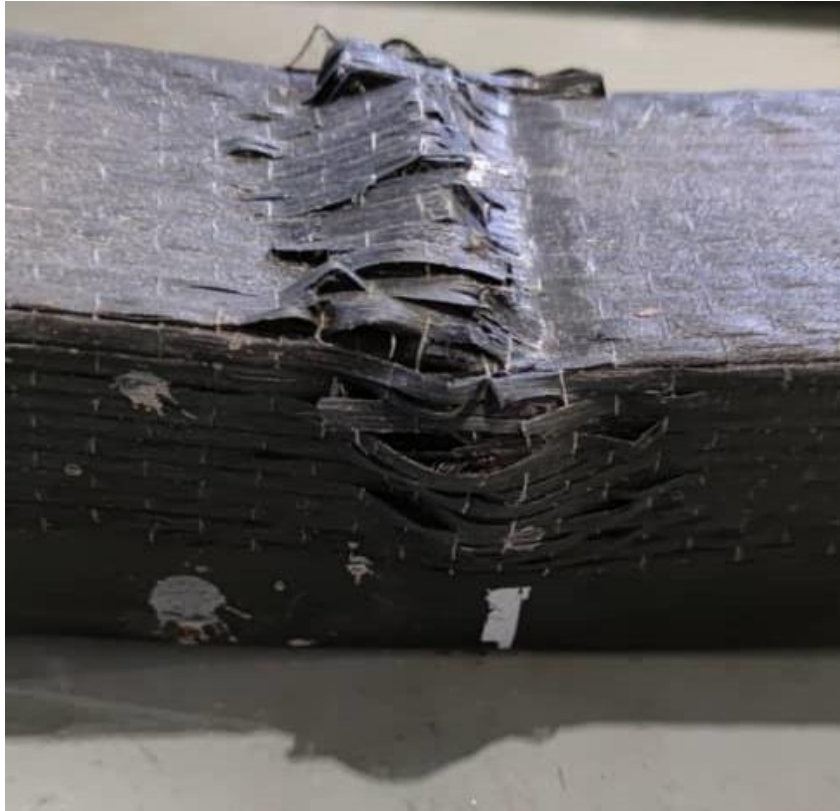
Figure 12 shows the CFRP rupture on CFST-2L
