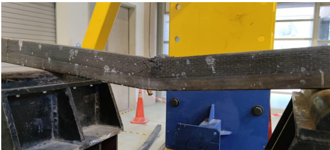
Figure 11 shows the buckling failure of CFST-3L
