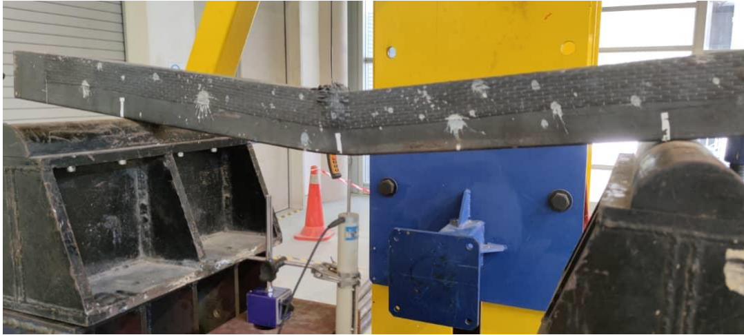
Figure 10 shows the buckling failure of CFST-2L
