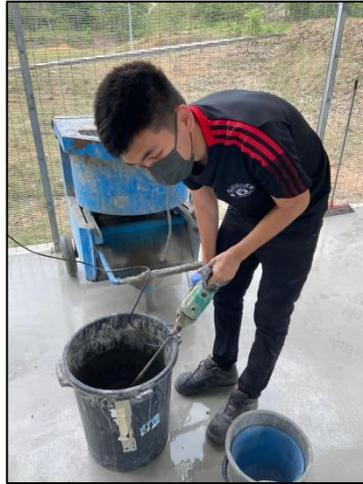
FIGURE 3.3: Mixing of GNP Cement Mortar by Portable Cement Mixer with Rod
