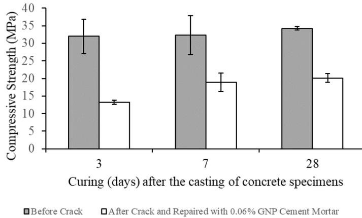
FIGURE 4.6: The Graph of Compressive Strength (MPa) against Curing (days) after Casting of Concrete Specimens
