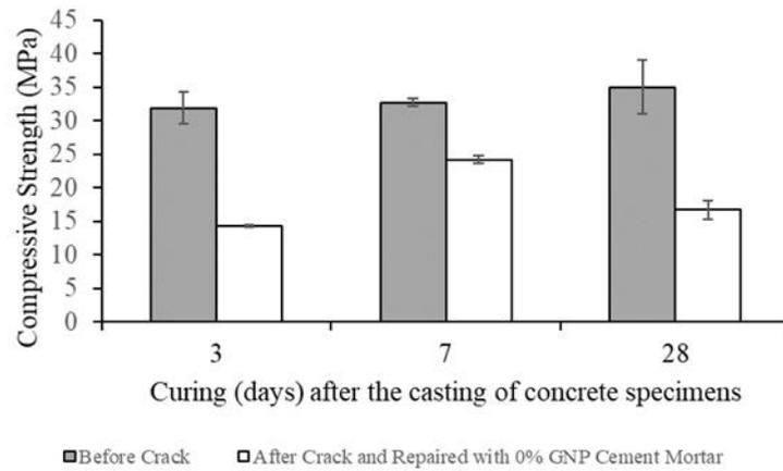
FIGURE 4.3: The Graph Compressive Strength (MPa) for those particular concrete specimens against Curing (days) after Casting of Concrete Specimens
