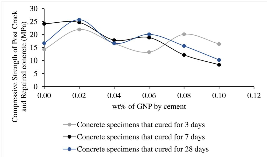
FIGURE 4.10: The Graph of Compressive Strength of Post Crack and Repaired Concrete (MPa) against wt% of GNP by Cement
