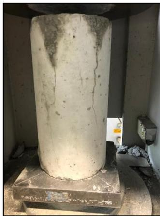
FIGURE 3.4: Testing of Compressive Strength for Post-Crack and Repaired Concrete Specimens
