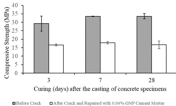
FIGURE 4.5: The Graph of Compressive Strength (MPa) against Curing (days) after Casting of Concrete Specimens
