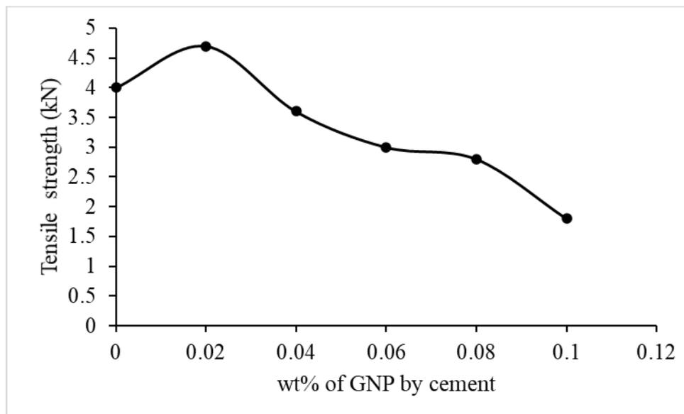
FIGURE 4.11: The Graph of Tensile Strength (kN) of Cement Mortar against the wt% of GNP by Cement
