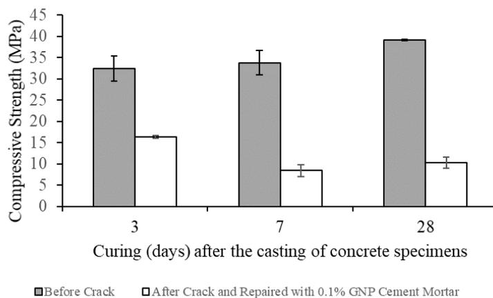
FIGURE 4.8: The Compressive Strength (MPa) against Curing (days) after Casting of Concrete Specimens
