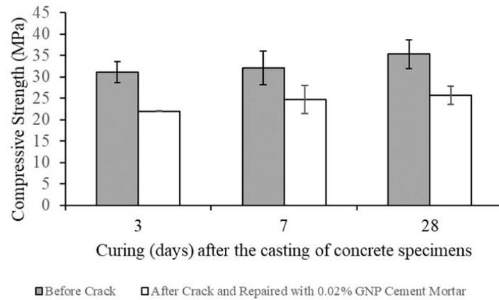
FIGURE 4.4: The Graph of Compressive Strength (MPa) against Curing (days) after Casting of Concrete Specimens
