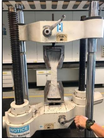
FIGURE 3.5: Testing of Dog Boned Shaped GNP Cement Mortar
