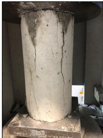
FIGURE 4.9: The Propagation of Crack from the Original Fracture Tips
